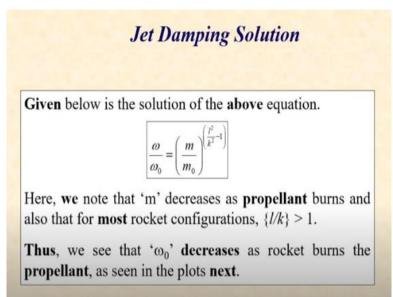
We can apply the simple formulae of integral calculus and we can show that  $\frac{\omega}{\omega_0}$  where,  $\omega_0$  is the initial angular velocity acquired at time t equal to zero is nothing but  $\frac{m}{m_0}$ , where  $m_0$  is the mass of vehicle at that instant of time raised to the power  $\frac{l^2}{k^2} - 1$ . And then we note couple of things with regard to the solution.
