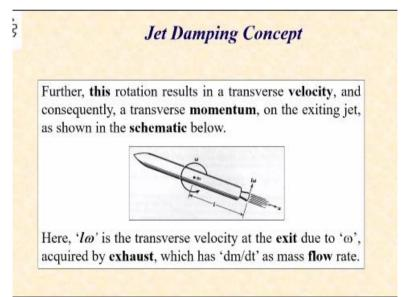
Now as vehicle rotates about its axis its front and back execute rectilinear motion and in the process, the jet which is exiting from the rear of the rocket acquires apart from the axial velocity due to burning of the propellant also a transverse velocity due to the angular velocity disturbance. The phenomenon is shown schematically below.
