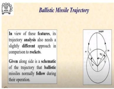
Let us look at these in a schematic that is shown alongside wherein we launch a missile and it is supposed to have an impact on the surface of the earth. So, in this we assume that there is an altitude point represented by burnout *bo* where the missile is given a velocity with which it starts traveling in the gravitational field of earth.
