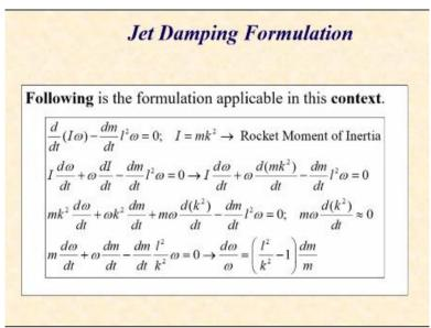
Following is a basic formulation applicable in this context. So let us start with the angular moment balance equation. So, the rate of change of angular momentum  $I\omega$  is to be balanced by the torque which is applied and as this torque is in direction opposite to the inertia torque, we have this equation. And as there are no other external moments acting on it, the right-hand side is zero.
