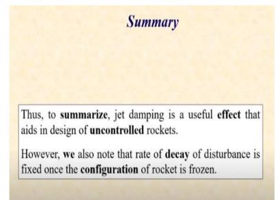
So, to summarize, jet damping is a useful effect that aids in design of uncontrolled rockets. However, we also note that rate of decay of disturbance is fixed once the configuration for rocket is frozen.
