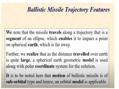
It is generally found that the best possible trajectory that such a missile can take is a segment of an ellipse which provides directly the impact point from geometric relations of the ellipse. Of course, we realize that as the distance traveled over earth is quite large, the flat earth the model that we commonly employ in the context of launch vehicles or rockets is not really applicable.
