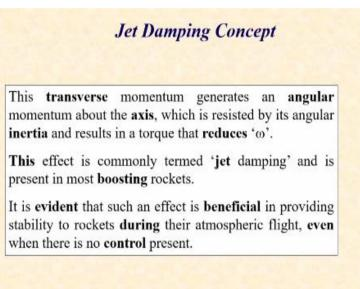
Now this transverse velocity has a transverse momentum and rate of change of that transverse momentum generates a transverse force which is nothing but  $\dot{m}l\omega$ . And now this force tries to generate a moment about the axis which is  $\dot{m}l^2\omega$ . Now this moment as we all know from our Newton's laws is resisted by its angular inertia such that there is a resistance to this motion which reduces  $\omega$  as time progresses.
