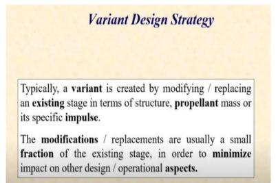
So, this brings us to some discussion on the design strategy. So how does one do this exercise or how does it happen? Typically, a variant is created by modifying or replacing an existing stage in terms of either structure or propellant or its specific impulse. For example, you might still be using the same stage I of PSLV. May have the same mass for propellant, but you may pack it with a propellant which is maybe a slightly higher  $I_{sp}$ .
