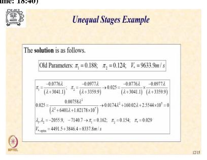
So, the old parameters if you remember you can go and check the  $\pi_1$  was 0.188 the  $\pi_2$  was 0.124 and corresponding to these two the  $V_*$  was 9,633.9 m/s. This was the solution that we
