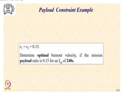
Let us now flip the problem and look at when we want to put a payload constraint and see what is the solution that we get and what is the velocity that we are going to get. So, in the previous case the payload fraction that we had got was 0.106. Let us try for a slightly higher payload fraction of 0.15 and let us see what happens to the solution for the same set of structural ratios and same  $I_{sp}$  of 240.
