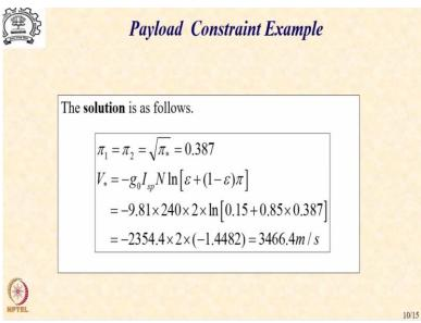
So, this solution is as follows. Now we know that both the  $\pi$ 's are same which are nothing, but  $\sqrt{\pi_*}$  sand it is 0.387. So, now you can see in the previous case the  $\pi$  was 0.32, but now the  $\pi$  has become 0.38. So, the payload ratios are higher because the payload ratios are higher now, I substitute these into my  $V_*$  expression and what I get as  $V_*$  is slightly lower.
