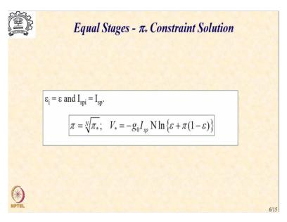
Let us look at the same thing for  $m_*$  or  $\pi_*$  constraint. So, in this case because  $\pi_*$  is a constraint it can be shown that all the  $\pi$ 's will be same because all the  $\pi$ 's are same the  $\pi$  will be nothing, but the  $\sqrt[N]{\pi_*}$ . So, directly that is the solution for a stage payload ratio and the  $V_*$  now can be obtained directly from this value of  $\pi$ .
