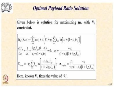
Let us now look at the counter part of this particular solution where we would like to maximize  $m_*$  or in this particular case the  $\pi_*$  the payload fraction with  $V_*$  as the constraint. So, in this case we use the augmented objective function  $H_{\pi}$  where the first term that is  $\sum_{i=1}^n \ln \pi_i$  is the objective part coming from the  $\pi_*$  and then we have the constraint error multiplied by the Lagrange Multiplier  $\lambda$ .
