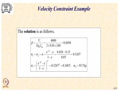
So, the solution is as follows. Let us go through the steps one by one. So, let us first calculate  $\beta$  which is  $\frac{V_*}{Ng_0I_{sp}}$  as it is a two stage it is 4,000 which is the  $V_*$ ;  $\frac{4000}{2\times9.81\times240}$ . So, we get a  $\beta$  value of 0.8494. Substituting this into the expression for  $\pi$  which is  $\frac{e^{-\beta}-\varepsilon}{1-\varepsilon}$  we get  $\pi_1$  as 0.3267. Now this is the value which is common for both the stages.
