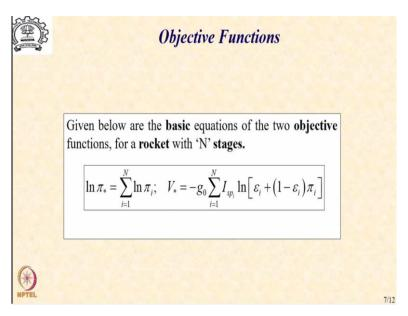
So, as you recall we had given two scenarios in the context of multistage rocket design. The first one was that we would like to maximize the burnout velocity for a specified payload constraint or we would like to maximize the payload for a given burnout velocity constraint. Let us now see what will happen to these two scenarios from the constraint optimization point of view when we make use of the Lagrange Multiplier and add the constraint error.
