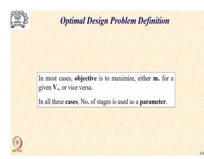
Now, we have already mentioned that we would either like to maximize the velocity for a given payload mass or maximize the payload mass for a given velocity. These are going to be our formal design objectives for designing a multistage rocket. Of course, it is important to take note of the fact that number of stages is strictly speaking an unknown and along with the stage wise mass parameters this can also be used as an unknown to arrive its value through the same optimization procedure.
