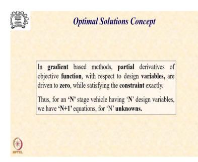
So, how does this gradient based method work? In gradient based methods, what we try and do is to generate the partial derivatives of the objective function with respect to all the design variables and from the basic understanding of calculus you would note that an optimal solution would be obtained when all the partial derivatives are zero at a single point. So, we now get as many numbers of equations as there are number of design variables which will be algebraic equations.
