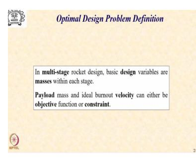
As we have already seen in multistage rocket design, basic design variables are masses within each stage. Further, we have also noted that there are two requirements from mission perspective that is the payload mass and the ideal burnout velocity and in a generic mechanism we can either use payload mass as a constraint. And try to maximize the ideal burnout velocity or we can put a constraint on the ideal burnout velocity.
