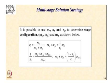
Let us make use of  $m^*$ ,  $\varepsilon_i \& \pi^*$  to determine the stage configuration which is meant by the  $m_{si}$ and  $m_{pi}$  for each stage as well as the total lift off mass in the following manner. So, let us first take the expression for  $\varepsilon_i$  which is written as  $\frac{m_{si}}{m_{si}+m_{pi}}$ . Now, let me do a little bit of algebraic jugglery and that gives me  $m_{si} + m_{pi}$  as  $\frac{1}{\varepsilon_i} m_{si}$ .
