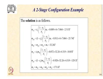
So, let us start the process let us go through it step by step. So, we start from the second stage because that is the last stage and  $m^*$  is known to us. So, I calculate  $m_{s2}$  as  $\varepsilon_2 \times \frac{1-\pi_2}{\pi_2}$  into  $m^*$ . I perform this simple arithmetic and I get this structural mass of second stage is 2.51 tons. Similarly, I use the  $m_{p2}$  expression and I get the propulsion mass as 25.74 tons. Now my starting mass for the second stages  $m_{p2} + m_{s2} + m^*$ .
