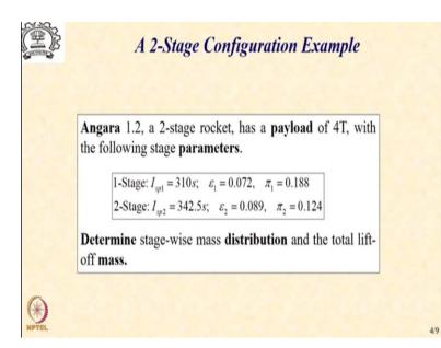
Let me demonstrate this through an example of a rocket which is in literature you can look it up called Angara 1.2 it is a two-stage rocket which is supposed to launch a 4-ton payload and has the following stage parameter as per our solution methodology. The first stage has the propellant with  $I_{sp}$  of 310s. Of course, for this exercise it is not really required, it has a structural ratio of 0.072 or what I call 7.2% structural mass.
