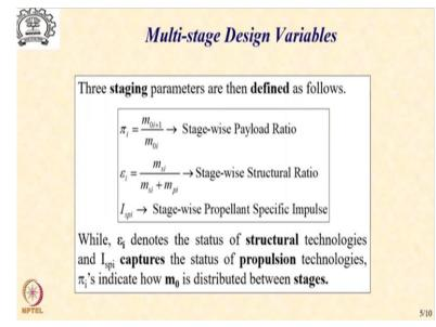
Based on this, let us now define the applicable design variables for a multistage configuration. So, let me introduce a parameter called  $\pi_i$  name stage wise payload ratio which is nothing, but the ratio of the payload of the  $i^{th}$  stage and the starting mass of the  $i^{th}$  stage. You may immediately connect this with the basic definition of the payload ratio that we have already used for the mission which is defined as  $\frac{m^*}{m_0}$ .
