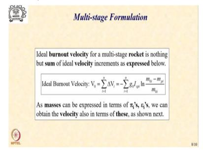
So, how do we set up this problem? The ideal burnout velocity for multistage rocket is nothing, but the sum of the velocity increments given by each of those stages. Each of those stages at an ideal  $\Delta V$  and if I add all of these the total is nothing, but the ideal burnout velocity that I will get from this multistage rocket. So, I can express this in terms of the parameters that I have defined as follows.
