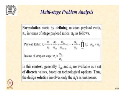
So, how do we formulate this problem? We formulate this problem by defining mission payload ratio  $\pi^*$  which is  $\frac{m^*}{m_0}$  and there is a constraint that this particular ratio has to obey in terms of the stage payload ratios that we have defined in the following manner. So, we defined  $\pi^*$  as  $\frac{m^*}{m_0}$  and then it is not very difficult to see that we can define a recursive process as shown through this multiplication until we arrive at  $m_{01}$ .
