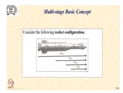
In this context, let us consider the following configuration that captures the spirit of a multistage rocket that we may have. In this picture, you note that the complete rocket has been divided into segments with the subscript 1 and 2 called the stages and the final payload module given a subscript  $m^*$ . Now, within each of the stages which is further subdivided into two parts, the propulsion and the remaining structure.
