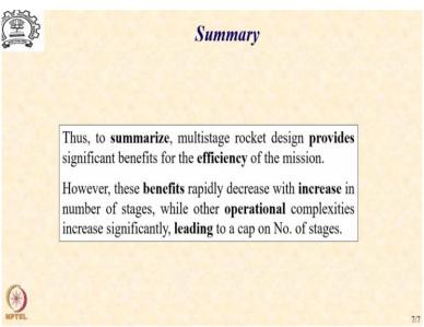
So, to summarize the multistage rocket design provides significant benefits in terms of energy or velocity and also very high efficiency of conversion of the propellant energy to the mechanical energy. However, these benefits rapidly decrease with increase in number of stages. While the operational complexities increase and results in a cap on the number of stages that are commonly employed for most practical launch vehicle to between three and four stages.
