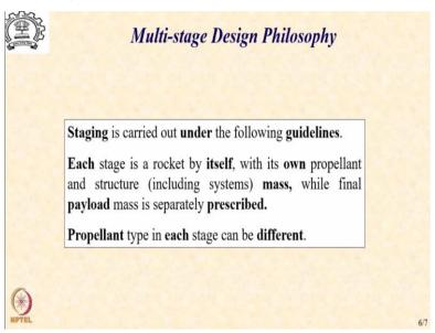
So, let us now understand the broad framework and philosophy within which the staging operation is going to be carried out. So, let us recall and each stage is a rocket by itself with its own propellant and structure including systems and mass which is altogether termed inert mass. While the final payload mass is separately prescribed as  $m^*$  as we have seen in the examples.
