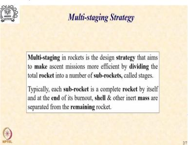
So, multi-staging in rockets is the design strategy that aims to make ascent missions more efficient by dividing the total rocket into a number of sub-rockets called stages. Typically, each sub-rocket is a complete rocket by itself and at the end of the burnout of the sub-rocket, shell and other inert mass are separated from the remaining rocket. This is the fundamental idea of the staging that you divide the total rocket into smaller segments.
