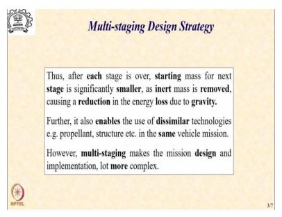
We see that the starting mass now for the next stage is significantly smaller as the inert mass which we were carrying earlier we are no longer carrying and we are throwing it away and this obviously means that the remaining propellant which is in the other stages which have not yet operated will need to accelerate a smaller mass and hence they will become more efficient from the overall loss point of view.
