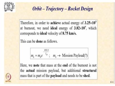
If we put these together, we find that in order to achieve the actual energy of 3.25 into 10 to the power 7 per unit burnout mass please note it's for unit burnout mass. We need ideal energy which is 15% to 20% higher than this. So, it is a 3.82 into 10 to the power 7. Now from our understanding of the ideal burnout we can immediately convert this energy as  $\frac{1}{2}V^2$  into the velocity which is ideal.
