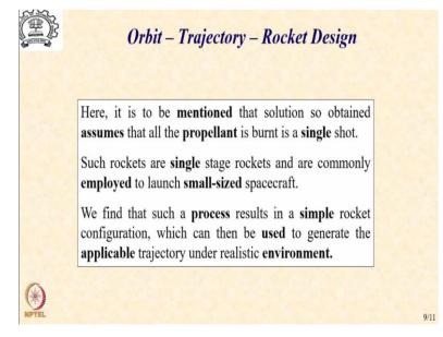
But there is another aspect that we now need to bring in before the solution becomes kind of complete. The equation that we have seen previously assumes that once you start burning the propellant you do not stop until all the propellant is consumed or that you are burning the propellant in a single shot. Such rockets are called single stage rockets and are commonly employed to launch small size space craft.
