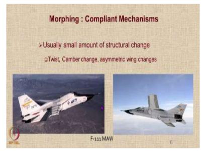
Similarly, when you go for compliant mechanisms, you usually go for these when there is a small amount of structural change, like when you want to have twist or camber change or an asymmetric wing change. So an example of this is F-111 mission adaptive wing which I already spoke about, that used compliant mechanism.
