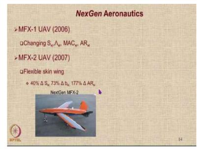
The MFX-2 UAV which came the next year, it had a flexible skin wing. It was seen that around 40% change in the wing area, 73% in wingspan and 177% in the aspect ratio was obtained in this particular aircraft.
