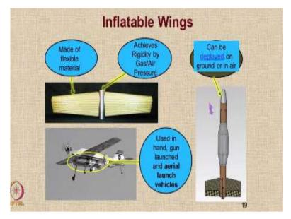
So as I mentioned, this is an example of inflatable wings. They are made up of flexible material and they achieve rigidity by gas, air, or air pressure, okay. You can use it in hand or gun launched and aerial launch vehicle such as this one which is mounted below this UAV. And they can be deployed on ground or air.
