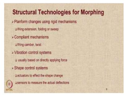
We also have variable camber, okay. In variable camber such as this aircraft, the F-18 Super Hornet, you can actually change the camber of the wing to desired value at various mission segments. But this experiment was ultimately not very successful and it was concluded that the cost and complexity and the weight because of the morphing on a big aircraft like this by variable camber is more than the benefits.
