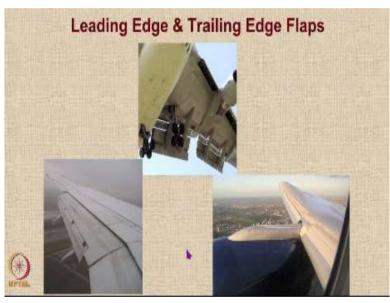
You can see these are the flaps which are the surfaces mounted on the trailing edge of the aircraft. This is another view of the flaps. You can see that not only do they deflect downwards they also create gaps between them. These are called as slotted flaps okay. And there are also flaps in the leading edge, the leading edge flaps as you can see this aircraft the leading edge flaps are deflected downwards.
