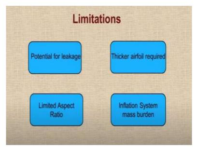
But there are also some limitations. One is there is a potential for leakage because it is inflatable structure. You require a thicker aerofoil because you cannot have very thin and sharp edged aerofoils with inflatable wings. The aspect ratio is limited because you cannot make it very slender because the air pressure will not then equally distribute towards the edges.
