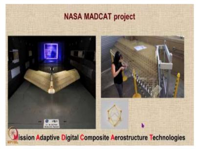
NASA is currently working on a project called as a MADCAT project which stands for mission adaptive digital composite aerostructure technologies. In this particular project, which is being done at MIT and California University. So you can see that the wing is consisting is created through an assembly of various small structures like this. And at the nodes, we have some sensors, okay.
