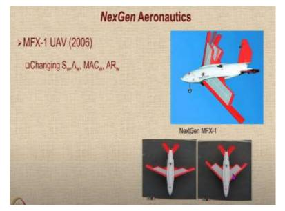
There is a company called NexGen Aeronautics which has experimented with morphing on small UAVs. The MFX-1 UAV as you can see on the screen was to change the wing area, to change the wing sweep, mean aerodynamic chord and the wing aspect ratio. And also it had asymmetric morphing as you can see only one wing is changing its sweep.
