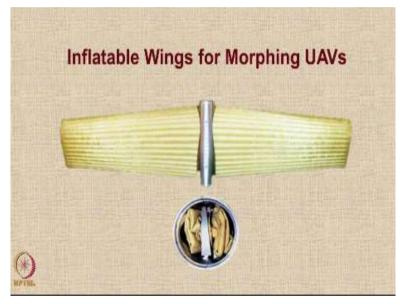
Let us move on to one special example of morphing which is inflatable wings for UAVs, okay. So here the wing is packed inside the fuselage like this so that you can launch this UAV like a barrel or like a small rocket kind of a thing. And then when needed, the wings will come out after they are inflated.
