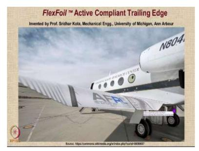
Now this is an example of a project which has gone from conceptualization in 1998 to actual testing on an aircraft in around 2015, I think. So this is the FlexFoil active compliant trailing edge, which was invented by Prof. Sridhar Kota of mechanical engineering department of University of Michigan Ann Arbor. You can see here that the wing does not have any discontinued parts.
