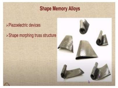
Shape memory alloys is one structural technology which is very useful in achieving morphing. Mostly it consists of piezoelectric devices and some kind of a, sometimes some kind of a truss structure. Here is an example of a shape memory alloy. So you can roll it and keep it in this condition for ease in transportation etc.
