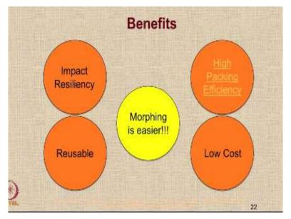
What are the benefits of inflatable wings? First of all, it gives impact resiliency to the aircraft. Many UAVs they break when they hit an obstacle during their flight. But in case of inflatable wings, probably you can make it very much resilient to impact. It gives you a high packing efficiency as an example.
