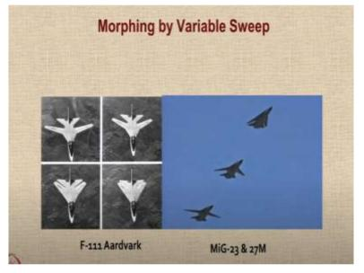
So variable sweep, here is an example of variable sweep in which the wing can have various positions. And in our own country, we have had experience of operating this aircraft MiG-23 and 27M. It also has got three specific positions at which the wing sweep can be created. There is a 16 degree 45 minutes position for the low speed flight takeoff and landing.
