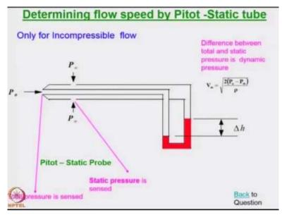
So this figure shows the working of the pitot-static tube. It shows that the tube has got a hole in the front which measures the total pressure and there are holes on the side which give you the static pressure. So when you calculate the difference between the total and the static pressure that is proportional to the square of the velocity. Hence
