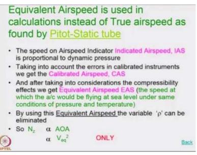
But the question is that the speed on the airspeed indicator is the indicated airspeed. Now that is proportional to the dynamic pressure which the air is facing. Is not the true airspeed, but if you take into account the errors in the calibrated instruments, then we get what is called as the calibrated airspeed and also the position. Now if you take care of the compressibility effects, then we get what is called as the equivalent airspeed.
