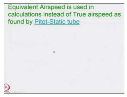
We do this by using equivalent airspeed in the calculations as against the true airspeed which the pitot-static tube normally determines.
