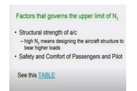
Now let us have a look at the factors that govern the upper limit of load factor  $N_z$ . The upper limit is decided based on the structural strength of the aircraft. High  $N_z$  means you have to design the aircraft to bear higher loads. But we have to also keep in mind that an aircraft will typically be carrying passengers and crew members.
