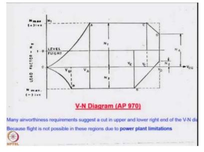
This is the V-N diagram as per aviation publication 970. So notice that in some airworthiness regulations, you are provided cuts or concessional zones in the right top and the right bottom area of the V-N diagram, because flight in these areas are not normally permitted because of the power plant limitations as we will see very shortly.
