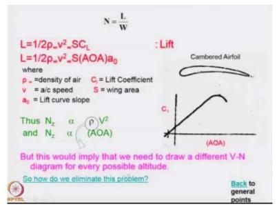
So the ratio  $N_z$  would be nothing but ratio of lift over weight. Now the lift is proportional to  $\frac{1}{2}\rho V^2 SC_L$ . And if we replace  $C_L$  by the angle of attack and the lift curve slope, you get S into AOA into  $a_0$ . So now if you take a ratio, so you will find that it will be proportional to  $V^2$  and also proportional to angle of attack a because for a given altitude rho infinity S and  $a_0$  remain constant.
