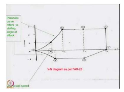
So here is a V-N diagram as per FAR part 23 regulations. We notice that there is a curve O to A, O being the origin with zero velocity and zero load factor. From O to A we have a parabolic curve and this parabolic curve corresponds to the stalling angle of aircraft because at this along this curve the aircraft has got the highest lift coefficient or the lowest speed.  $V_s$  corresponds to 1g stall speed or level flight stall speed.
