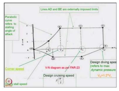
That is this value  $V_A$ . And then you have lines AD and BE which are externally imposed limits on the vertical positive and the vertical negative value of the load factor as prescribed in the table which we just now saw. Now this  $V_C$  corresponds to the cruising speed, the design cruising speed, which is a function of the wing loading of the aircraft W/S. And there is also another speed called as the design diving speed.
