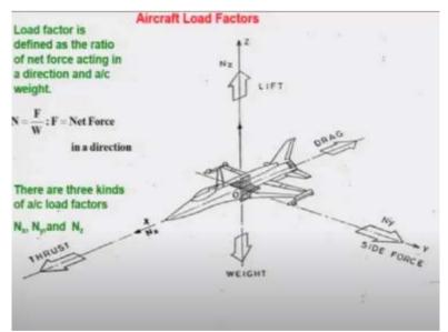
Let us see what is the meaning of load factor. A typical aircraft has three axes in which we define all the forces and moments. You have the vertical or the z direction in which the lift normally acts. We have the longitudinal or the x direction in which the thrust normally acts. And we have the lateral or the y direction in which the side force  $N_y$  normally acts. And the weight of the aircraft acts vertically below along the z axis.
