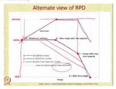
There is another way of looking at the range payload diagram which is if you plot on the x axis not just the payload, but the various weight terms, okay. So you see for example, that from the operating empty weight you include the payload and that then you hit the maximum zero fuel weight. So this is the limit on the maximum takeoff weight.
