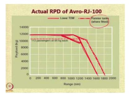
So let us see the actual payload diagram of an Avro-RJ-100. So this is the basic diagram, the dark red one. And when you install some additional fuel tanks called as the Pannier tanks, then you can increase the range by some amount, but still you then very soon you will hit the limit on the Pannier fuel tank also and then you can only travel further by reducing the payload, okay.
