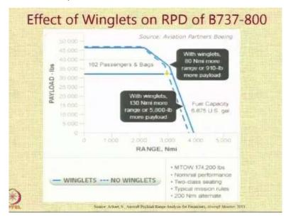
Let us see the effect of winglets on the range payload diagram of this Boeing 737-800 aircraft. Many companies are many airlines are installing winglets on the aircraft to try and improve its fuel consumption. So as this particular graph shows, if you install winglets, you get 80 nautical miles more range or you can carry around 910 pounds of higher payload for the same aircraft. And that happens in this particular regime.
