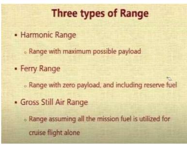
There is one range called as the harmonic range, which is just the range that we observed without compromising on the maximum possible payload carrying capacity, how much can you travel with the given amount of fuel tank okay, keeping some fuel for reserve. That is called as the harmonic range and this particular range is most important for an airline to know.
