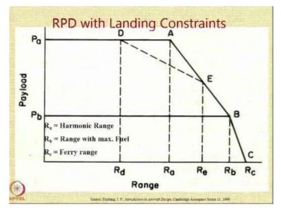
So this is what will be the range payload diagram with constraints on the landing weight. (**Refer Slide Time: 15:25**)
