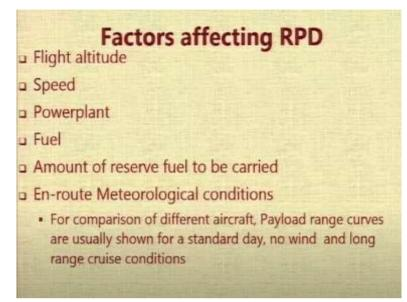
We are going to look at a detailed tutorial in which the calculations will be explained. Let us have a look now at some of the factors that affect the range payload diagram. The first factor that affects the range payload diagram is the flight altitude because at different altitudes the aircraft has a different specific range, okay. Then the speed. There is one speed at which the fuel consumption is minimum.
