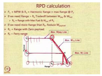
So the RPD calculation or the range payload diagram calculation thus is in terms of these three or four important points. The first point of importance to us is the point  $P_a$  okay. Now  $P_a$  basically stands for the payload that you know is the maximum payload and a is the harmonic point and range  $R_a$  is the harmonic range. So  $P_a$  basically stands for maximum payload weight.
