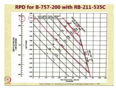
Here is a diagram that shows the effect of the limit on the takeoff weight. So there is a boundary diagram, there is the load diagram where you have the maximum zero fuel weight and there is a corresponding payload for it. Then this is the gross weight. Now in this particular line, the gross weight is 108.9 thousand kilograms, okay. And this is the maximum fuel line.
