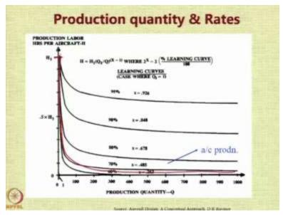
The production quantity and rates are also going to affect and this particular graph is generally called as the learning curve. So, the learning curve indicates that as you increase, as you produce more and more of particular items the cost per the production labor hours per aircraft are going to
