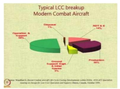
They have a huge lock-in the lifecycle cost. Here is a typical breakdown of combat aircraft, we noticed that nearly half the cost of the lifecycle is in operations and support and around 30% is in the production of the aircraft. The ground support equipment the initial spares can be around 5%. The design and development cost and testing costs could be around 14 to 15% and the disposal cost would be only about 1%.
