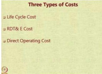
When we look aircraft conceptual design, there are 3 types of costs involved. The first one is the lifecycle cost or the LCC, the second cost is the RDT and E cost. And the third is the direct operating cost or DOC.
