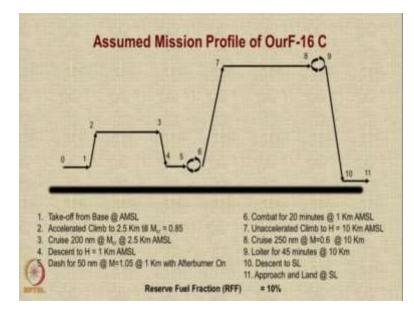
Let us have a look at the assumed mission profile of our F16-C aircraft. So, that is the ground the aircraft is expected to take off from a base which is located at mean sea level, it is then undergoes an accelerated climb to a height of 2.5 kilometers. The End Mach number of the accelerate climb is 0.85, so, from approximately 0.2 Mach number when it is at the end of the climb or at point number 1, it accelerates to Mach number 0.85 in an accelerated climb.
