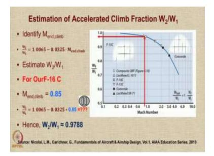
So, to calculate the fuel fraction in the accelerated climb, we first identify what is a Mach number at the end of the climb, then we use this equation to get the value if the climb is supersonic and if there is subsonic there is another formula available with that you estimate  $\frac{W_2}{W_1}$ . For our F16-C aircraft, the Mach number at the end of climb is 0.85 which is the cruise Mach number.
