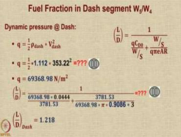
So, the value of q is available by multiplying by density and the velocity that is 69368 Newton per meter square and then you can estimate the L/D using this formula. So, putting in the numbers, so,
