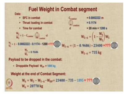
After that, we do a combat for 20 minutes. So, it is given that the SFC is 80 per hour or 0.0002222, thrust loading in combat is known from the previous initial sizing calculations, the time for combat is specified as 20 minutes or 1200 seconds. So, the weight fraction in the combat would be 1 minus SFC of the combat into T/W of combat into d. So, it turns out to be 0.9686. So, for the combat segment, once again the weight would be just 1 minus the ratio into the old weight.
