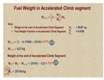
So, this is a standard formula for every segment, fuel consumed in a segment will be equal to 1 minus weight ratio at the beginning on another segment into the wait at the beginning of the segment. So, we know that for this aircraft, the weight at the start of the accelerated climb is what we got earlier as a weight at takeoff minus the fuel consumed during takeoff and warmer and we also know the value of fuel weight fraction. We have just seen it in the chart or done the calculation.
