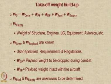
Let us look at the first step in refined sizing which is the takeoff weight built up. So, as per refined sizing procedure the aircraft weight is considered to be consisting of these elements, there is a crew weight, there is a fixed payload, and the droppable payload, there is a fuel weight and the empty weight. The empty weight consists essentially of the weight of the structure the engines the landing gear equipment, avionics etcetera.
