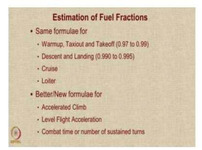
So, the formulae are the same for warm up taxi out and take off. The ratio also is similar the descent and landing crews and loiter the same formula, the difference is that there will be a much better formula for accelerated climb, level flight acceleration. And for the combat using the combat time or the number of sustained turns, we are going to get a formula to directly estimate the value of fuel.
