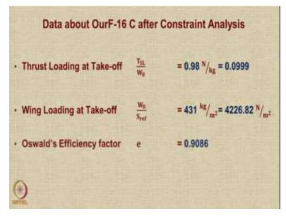
We also look at some data about our F16-C which we obtained earlier in the constraints analysis. So, we have obtained the thrust loading to be 0.98, and wing loading to be 431 kg per meter square we are converting them into dimensionless units and written in my meter square here for our calculations, Oswalds efficiency factor was determined using the aspect ratio and the Mach number as 0.9086. So, we keep it like this.
