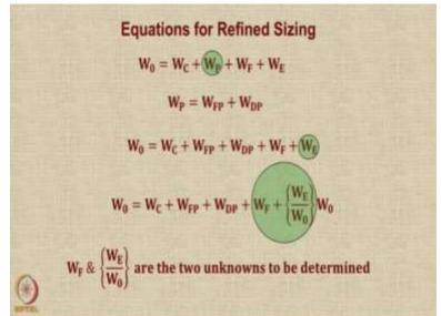
Let us look at the equations for refined sizing. So, once again  $W_0$  as a summation of these 4 components Crew, Payload, Fuel and Empty. For payload we have seen there are 2 terms of fixed payload and droppable payload. So, for empty weight we have empty weight fraction into  $W_0$ . So, it becomes an equation of iterative of nature because on the LHS we have  $W_0$ , on the RHS also we have  $W_0$  and this ratio is to be determined.
