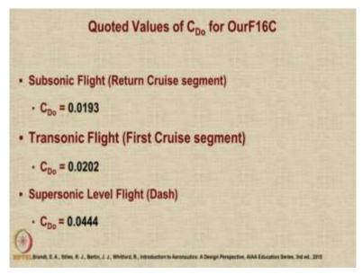
Then there are some quoted values of  $C_{D_0}$  for our F16 aircraft in the textbook by Brandt, Stiles, Bertin and Whitford for the subsonic flight that is Mach number 0.6 in the return cruise segment,  $C_{D_0}$  is given as 0.0193 for the transonic flight Mach number 0.85 which is in the first cruise segment, we are given  $C_{D_0}$  value as 0.0202. And for the supersonic level flight dash at Mach number 1.05.
