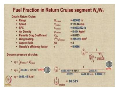
So, the range is 463000 meters that is 250 nautical miles, the speed is 179.66 that is from Mach number 0.6, the SFC is given as SFC cruise as 0.0002222 per second, the density of air at the altitude of 1.5 kilometer I assume would be 0.414 kg per meter cube the parasite drag efficient is 0.0193 because you are at a very benign low speed flight, and the wing loading as determined by the initial sizing for this segment is given.
