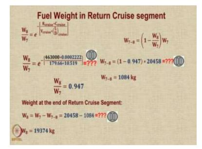
And the value of the empty weight fraction is obtained by the endurance equation in which  $W_8/W_7$  is 0.947. So, putting in the values in the formula, you can get the weight fraction as 0.947. And then the same formula applies even here. So, this is the weight fraction in this segment, and this is the weight at the beginning of this segment do calculate the value of  $W_7$  to  $W_8$  it is 1084 kgs.
