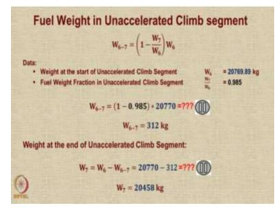
So once again the formula remains the same. But the data would be as follows the weight at the start of the climb is 20769.8 or 20770 actually, the fuel weight fraction in an accelerated climb is given as 0.985. So therefore, you can just put 0.985 in this expression and  $W_6$  in this expression
