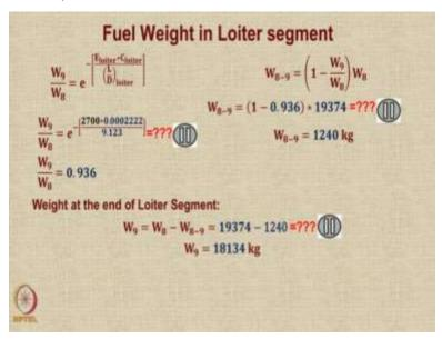
Now, Let us go to the loiter segment again we use the Bregeut range equation  $W_9/W_8$ , this is the equation for the weight remaining W 8 to 9 this segment, we are having a vacancy in weight. So, the value of the fuel consumed is 1240 kg, 20 minute loiter and a 10 kilometer altitude. So, the weight at the end would be 19374, which is the beginning of the loiter minus 1240, it is 18134. (**Refer Slide Time: 41:00**)
