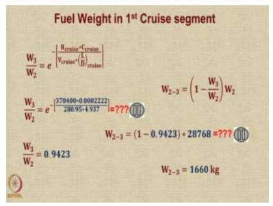
Fuel in the first cruise segment. So, once the ratio is known by inverting both sides, you can get
