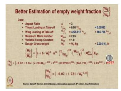
So, here is the formula. So, based on this formula and assuming that the aspect ratio is 3, the thrust loading is 0.98, the wing loading is 4226.817, Mach number as 2.05 and variable sweep constant is 1.0. You can estimate the Empty weight fraction value. Now, the design gross weight is not known, so it remains as it is so. So what we get is finally an expression. So, I think we need to calculate this expression. So, this is a place where you should pause the video and calculate these numbers.
