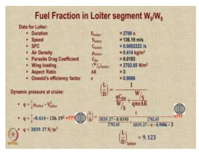
Finally, we come to the loiter segment at the end of the flight. So, for that we have been told that the loiter is happening for 45 minutes at the speed that we choose to be the optimum speed for the SFC would be 0.0002222 per second, density at 10 kilometer is 0.414, parasite drag efficient is 0.0193, Oswalds efficient factor is 2702.65 And finally, efficiency factor e is also needed in the calculation it is 0.9086.
