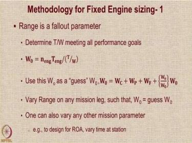
So, let us see what is the procedure to be followed for sizing when you do fixed engine sizing and when you do rubber engine sizing let us look at the fixed engine sizing first in the fixed engine sizing suppose you say that I am not particular about the range, range will be something that I get give me the performance then what you do is you first find out the T/W that meets all your performance requirements forget about the range.
