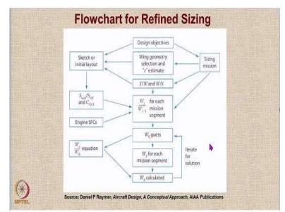
So, here is a flowchart for explaining the same procedure. So, you can see that there is a sizing mission from the mission we get the wing geometry and therefore, you can estimate the value of e from the sizing mission and sustain analysis we also know the value of T/W and W/S. So, from the sketch of the layout, you can get the wetted area ratio, you remember the graph given in Raymer's textbook where you eyeball the aircraft.
