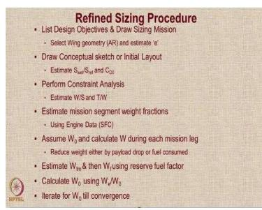
So, just to sum the refined sizing procedure, so, what you do is you list the design objectives and draw the sizing mission that is the mission profile you have to select wing geometry that means aspect ratio mainly and then you have to estimate the value of Oswald efficiency. Remember we had one very large big formula in terms of sweep of the maximum thickness line and the taper ratio etc. And aspect ratio mainly so, you can get the value of e.
