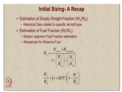
So, let us do a quick recap about initial sizing. If you have not watched the video lectures about initial sizing, I would recommend that you should go and do that before you proceed further. This is only a recap. So initial sizing, the first thing that we do is we estimate the empty weight fraction. For this if you remember, we use historical data related to specific aircraft type, we use the equation  $A * W_0^c$ .
