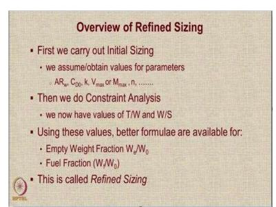
Let us first have an overview of refined sizing. So, first we carry out initial sizing we assume or obtain the values of certain parameters such as the wing aspect ratio, the aircraft zero lift drag coefficient  $C_{D_0}$  the induced drag coefficient k,  $V_{max}$  or  $M_{max}$  load factor n etc. Once we do initial sizing, we have an estimate of W<sub>0</sub> the design gross weight. And since we know the values of various constraints imposed.
