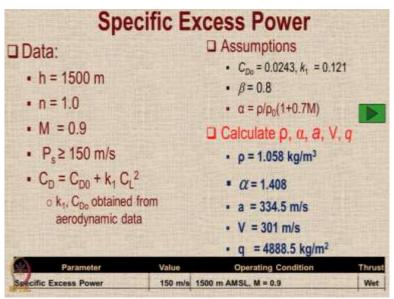
Moving ahead let us look at the specific excess power which is again specified in the constraints as shown in the line in the bottom. So, what do we see, we see that the height is 1500 meters, this is the level flight so, n = 1 the Mach number is transonic 0.9 and in this condition we want the specific power to be 150 meters per second or more the aerodynamic data is to be obtained from the information available.
