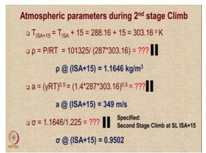
It is specified that the second stage climb occurs that ISA + 15 degrees. So, first thing to do is to calculate the value of the temperature at ISA + 15 degrees centigrade that is 288.16 which is the ISA temperature at sea level plus 15 degrees. And using this information we can calculate the value of density.
