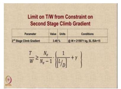
And we will start by looking at how the thrust to weight ratio is limited by constraints on these parameters. So, the first one is the second stage climb radiant as specified in the constraint table. The second stage climb gradient is expected to be 3.49% minimum when the aircraft is at the maximum takeoff weight of 215971 kilograms under ISA + 15 conditions at sea level. And to calculate this we will use this particular formula if this formula seems unfamiliar to you.
