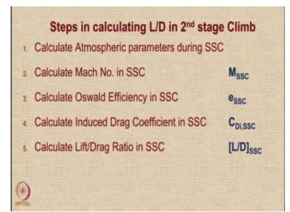
And let us see how we can calculate it. So, this calculation happens over I think 5 steps first, because the second stage climb is happening at ISA + 15 degrees, we need to do some atmospheric parameter calculation, then we calculate the Mach number in the second stage climb which we call it as  $M_{SSC}$ . Now, recall we have seen a formula to get the value of Oswald efficiency as a function of Mach number.
