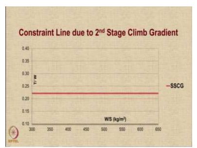
So, this appears as a single horizontal line because for there is no role of including in this case we got a direct constraint on T/W. So, the T/W value has to be always more than 0.2219. So, therefore, this is the horizontal line. So, the area which is shaded below this line is infeasible and the area above this line is feasible.
