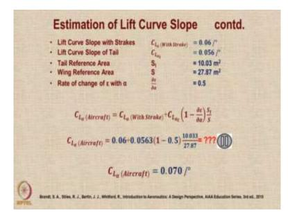
Moving ahead, so, we know the lift curve slope which takes as 0.06 we have just calculated the lift curve slope of the tail also as 0.056 the tail reference area was 10.03 meter cubes and we also know the wing reference area, and we are just calculated  $\frac{\partial \varepsilon}{\partial \alpha}$  of 0.5. So, therefore,  $C_{L_{\alpha}}$  for the aircraft will be  $C_{L_{\alpha}}$  with the strake which we have already calculated
