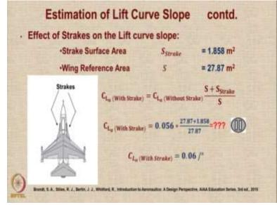
Let us continue ahead, we will like to look at what is the effect of strakes on the lift curve slope. Because as I mentioned, this aircraft is fitted with 2 strakes which are mounted at the wing fuselage junction ahead of the wing. These 2 strakes total area is 1.858 square meters, it was 20 square feet, and the wing reference area was 300. So it is 27.87 square meters. So the book by Brandt et al gives a simple formula for calculating  $C_{L_{\alpha}}$  of an aircraft with strake.
