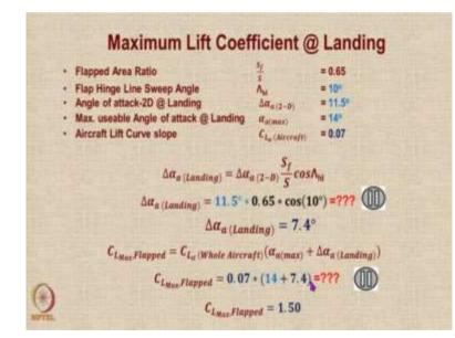
Let us repeat the same calculations for the landing condition during landing the geometrical parameters actually remain the same, the only change that happens is that the angle of attack 2D at landing because of the flaps in landing configuration is slightly higher because flaps are more effective in landing.
