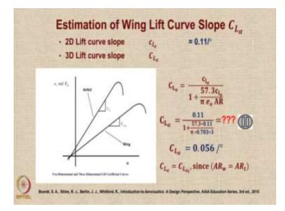
Let us now use this information to calculate the lift curve slope of the entire wing the so called 3D effects. So, the 2D lift curve slope we have just calculated was 0.11 per degree, the 3D lift curve slope will be called as  $C_{L_{\alpha}}$ . And here is a graph that shows how the  $C_{L_{\alpha}}$  of the airfoil and wing are different we notice that the wing has in general a lower lift curve slope compared to the airfoil.
