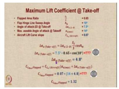
And that area is mostly the area inside the fuselage actually over the fuselage. So the flapped area issue is known as 0.65, hinge line of the flaps is swept at an angle of 10 degrees. From literature given in the textbook or you can say back calculated from some number in the textbook, we have determined that the angle of attack 2D at takeoff is 1.5 degrees. And as I mentioned to you the maximum usable angle of attack at takeoff is 14 degrees.
