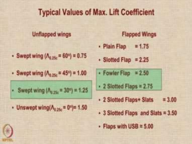
So before we go ahead with calculating the values of the maximum lift coefficient, let us get an idea about what are the typical values based on the literature that is available. If we look at unflapped wings, we see that wings with very large sweep of 60 degrees or so, they have a very
