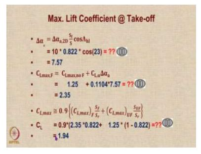
So, using these, let us start calculating the max lift coefficient at takeoff condition. The formula is as shown on the screen; we need to get the parameters  $\frac{S_f}{s} \cos \Lambda_{hl}$ . So we already know that this number is 10. This ratio we have already calculated as 0.822 and  $\cos \Lambda_{hl}$  as well also we took out the maximum of the both, so pause your video here and try to calculate delta alpha the value turns out to be 7.57.
