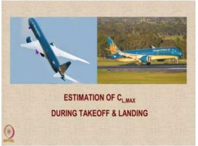
Let us now try to estimate the  $C_{L_{max}}$  value for this aircraft during takeoff and during landing. We see on the screen 2 pictures of the Vietnam airways Vietnam Airlines Boeing 787 aircraft just after takeoff in a very steep climb, very clearly showing the working of the outboard flaps and the inboard flaps. And here we have the same aircraft when it comes into land.
