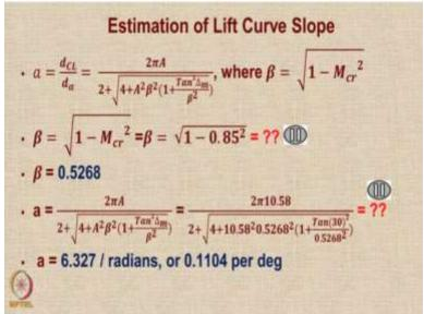
Let us first start with estimation of the lift curve slope for which we will use this formula where *a* is equal to
