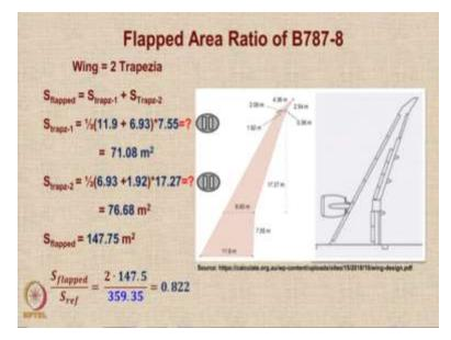
Now let us look calculate the flapped area ratio of Boeing 787-8. So here is the same wing. Once again I show you the wing but only half the wing is shown and this particular wing can be replaced by a series of geometrical constructs. Incidentally, the flapped area would consist of 2 trapezia, the first trapezium would be the one that goes from the root to the mid span break and the second trapezium would go from the mid span break to almost the wing tip portion.
