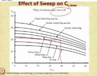
This graph from Raymers textbook shows 2 things. It shows that different flaps types have higher values of  $C_{L_{max}}$ . And it also shows how these values reduce with the increase in the quarter chord sweep. So you can use this graph for the wings of moderate aspect ratio only. And with this graph, you know you can probably get something like if the sweep is 40 degrees, and the flap type is
