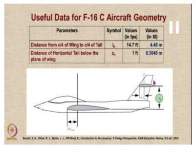
We also need some data from the side view for example we need the distance from the quarter chord of the wing to the quarter chord of the tail the so called tail arm and we also need the value of the lateral or vertical displacement of the horizontal tail from the plane of the wing which is 1 feet 0.3048 meters in this case.
