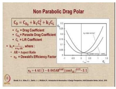
Many aircraft have a non parabolic drag polar here is an example. So the C D for such aircraft can be expressed in terms of
