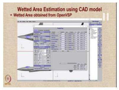
So using this particular CAD model it is possible to actually get the wetted area and also the parasite drag coefficients directly in the software.
