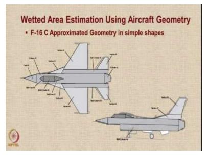
And then what we do is we approximate the geometry in simple shapes. So for instance you have three view of the aircraft. So you can see that in the top view you just create some simple surfaces and also in the side view you also try to create some simple surfaces try our best possible to match the geometry with that given and then you can do rendering of those surfaces to remove the internal details and hence you can get some idea about the various components.
