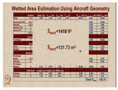
The value of  $S_{wet}$  given is 1418 square feet and spread calculated is 131.73 by converting this number. So what has happened is throughout in these calculations we have done rounding off because each quantity given in feet has been converted into meters rounded off and used in the calculation that is why there was an error of approximately you know eight and a half in 130.So we will go ahead assuming this to be the value because we do not want to introduce errors unnecessarily
