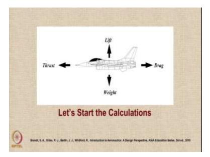
So let us start the calculation for an aircraft in level flight where all the four forces are in balance but while operating at a cruise mach number so we are going to go through calculations at cruise mach number under the ISA.
