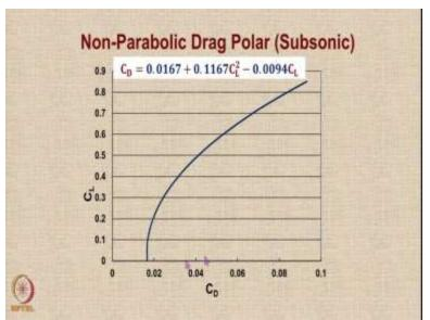
So when you plot this polar this is how you get so not very apparent but it is clear that this polar is not having the minimum at  $C_L=0$ . There is a shift in the  $C_L$  and this is the formula.
