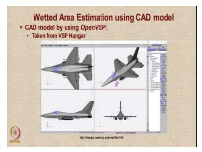
So we have done the same thing. So first we looked at CAD model by using open VSP and we took a model available from the VSP hangar this is that model but if you notice this model has these 2 bombs already loaded and also these 2 additional missiles loaded. So we do not need this. So this is how you render the shape of the model.
