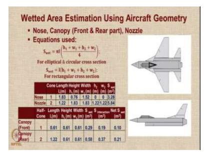
Moving ahead if you look at the nose the canopy front and the rear part because the mid part is a cylinder and the nozzle we get cones or frustrum of the cones and for that we can use standard formula available. So nose can be considered to be conical and with a nose cone of length height and width the end and the rear portion can be a frustum of a cone. So there are 2 cones here with  $l_1,h_1,w_1,h_2,w_2$  then for the canopy front it is half cone or a small cone.
