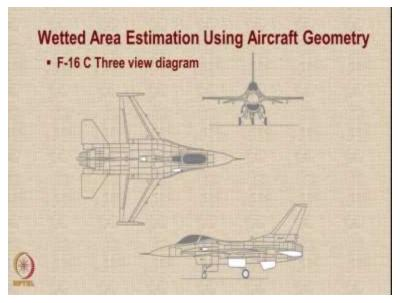
Now let us look at the second method where we look at the aircraft geometry and convert that into standard simple shapes. So here is a 3 view diagram of the aircraft.
