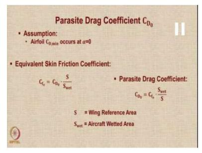
So for that we have to make some assumption. So we assume that this minimum drag occurs the airfoil has a minimum drag at  $\alpha = 0$ . And we look at the equivalent skin friction coefficient that will be
