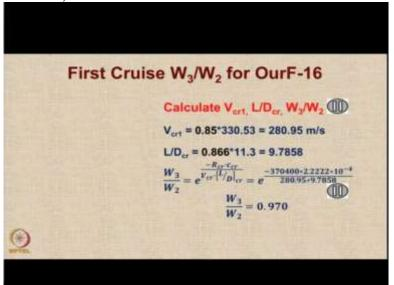
So, now I think we should, we have enough data to calculate the values of the cruise velocity, L/D cruise, and the weight ratio in the cruise. So at this stage, I would request you to pause the video and do these calculations. Let us see the values. So the cruise speed is 0.85 specified the Mach number into 330.53 that is 280.95. The L/D will be 0.866 times 11.3 which is the maximum L/D that is 9.7858.
