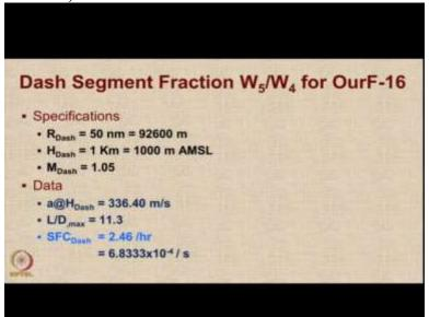
The dash segment is a segment in which we are going to travel just 50 nautical miles, 92.6 kilometers, but it is going to be at a supersonic mach number of 1.05. So under this condition, of course, the value of a can be calculated this is almost known to us the L/D max is 11.3 and SFC you will notice is 3, more than 3 times that of the cruise. So keeping these numbers in mind,
