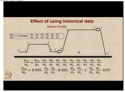
So as I mentioned, the warm up takeoff and landing weight fractions are estimated by historical trends and fuel consumed and the distance travelled during different segments is completely ignored. Effect of using historical data, this is our basic mission profile. And these are the 10 segments for which we had to estimate the mission segment weight fractions. But we can use historical data for this 0.97 corresponds to the warm up, taxi out and take off.
