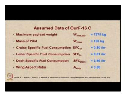
So, we will assume some data for Our F 16 C aircraft. The maximum payload weight is assumed to be 7575 kgs. This is similar to the maximum payload of F 16. The mass of the pilot along with the g suit is assumed to be 100 kgs, 75 kgs for the pilot 100 kgs total with all the paraphernalia, with the helmet et cetera et cetera. The SFC of the aircraft, the single engine aircraft in cruise is 0.8 per hour and the loiter specific SFC would be slightly more 0.81per hour.
