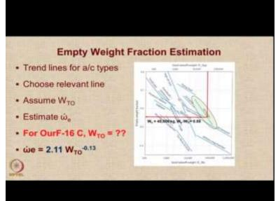
In our case, what we do is we look at these trend lines for various aircraft types. And we choose the relevant line for us it is jet fighter, and we assume some  $W_{TO}$ , and then come onto this line, and then we estimate the empty weight fraction by moving horizontally. So for example, if we assume the max takeoff weight to be, the size takeoff weight to be 45000 kilograms. For a jet fighter, it turns out to be approximately 0.55 as the empty weight fraction.
