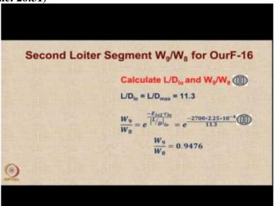
And then we have the second loiter segment which occurs for 45 minutes, for this the data is the same. And the L/D also is going to be the same, L/D max, we just need to do the calculation by putting in the correct value of the duration of our loiter in this expression. So this number, you can pause the video and do the calculation. The number turns out to be 0. 9476.
