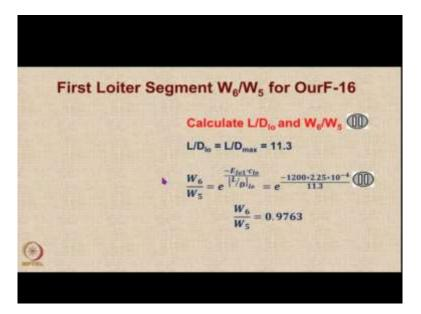
So, for the first loiter segment for Our F 16 aircraft, we have the requirement of 20 minutes of endurance which is 1200 seconds, the data is L/D max is 11.3, SFC is given as 0.81 per hour. And now we can calculate L/D during loiter and the weight ratio. The L/D is going to be the same as L/D max as I already mentioned, and for the weight ratios, we just have to do the calculation using this expression. Pause the video and do the calculations please. We get the weight ratio is 0.9763.
