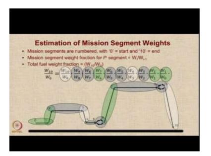
So, we can use the method. So, what we do is we number the mission segments from 0 to 10 in this case. And for any i<sup>th</sup> segment, for any segment, so if there are 10 numbers there will be actually 9 segments. So, for any segment the fuel weight fraction would be  $\frac{W_i}{W_{i-1}}$ . The total fuel fraction would be  $\frac{W_{10}}{W_0}$ , which will be obtained as a simple multiplication of the fuel weight fraction in each of these segments.
