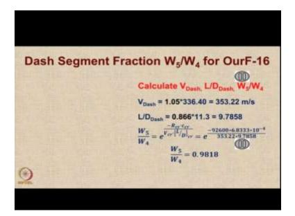
let us calculate now the value of  $V_{dash}$ , L/D dash and the weight ratio. So, I would like you to pause the video and do the calculation.  $V_{dash}$  will be simply mach number into sonic speed. Remember there is a slight difference because we are assuming conditions to be changing. It is not just ISA conditions. L/D dash will be again it is a cruise, so it will be 0.866 times L/D max and for the weight ratio we will have a formula.
