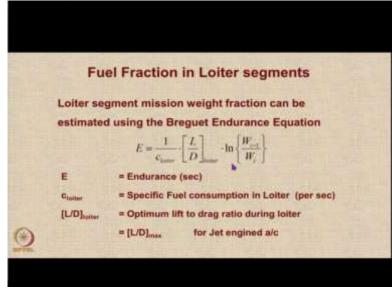
Now, we go to the 2 loiter segments, again you can use the Breguet endurance equation, but here the c will be the c for loiter which is in this case given us slightly more than that for cruise and L/D loiter was going to be L/D max because it is a jet engine aircraft and we know that jet engine aircraft obtains its max endurance when it flies at a speed corresponding to L/D max. (**Refer Slide Time: 25:53**)
