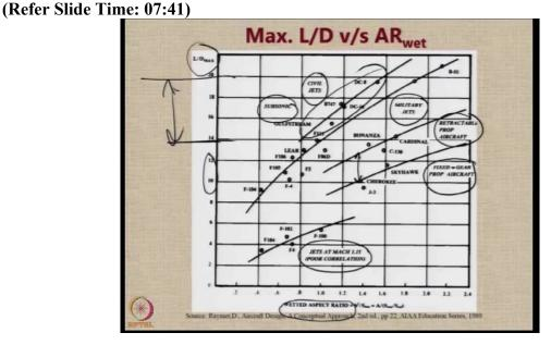
So, this way, you can use this particular chart to get a ratio of what is the typical expected value of  $\frac{S_{wet}}{S_{ref}}$ . And then there is another chart where the wetted aspect ratio on the x axis. This is the wetted aspect ratio that means span square by the wetted area, this is plotted and on the y axis you have the expected value of  $\left(\frac{L}{D}\right)_{max}$  and there are lines for various aircraft types.
