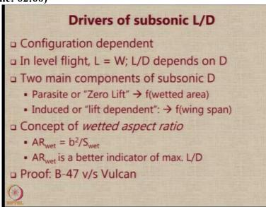
Let us understand what are the drivers of subsonic  $\frac{L}{D}$ ? The subsonic value of  $\frac{L}{D}$  is very strongly dependent upon the aircraft configuration. In level flight, we go for a condition that lift is equal to weight and hence, the  $\frac{L}{D}$  will depend based mostly on the D because the L is
