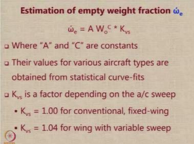
A and C are constants which are a function of a particular aircraft type, their values are obtained by a statistical fit of existing data  $K_{vs}$  is just a multiplication factor that tells us the effect of providing variable sweep. So,  $K_{vs}$ = 1.04 basically tells us that if you provide variable sweep in a aircraft, which you would probably never provide in the transport aircraft, then you have to have a weight penalty of 4% of the total weight.
