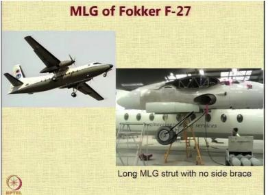
Here is the main landing gear of the Fokker F-27 aircraft which is now obsolete. It had long main landing gear struts with no side braces. So, these were the landing gear struts which are quite long because it was mounted on the wing and the wing was a high wing. So on a high wing aircraft, where the wing is above the fuselage when you mount the landing gear of course they mounted it below the engines, but still it was an example of a long main landing gear stuck with no side braces.
