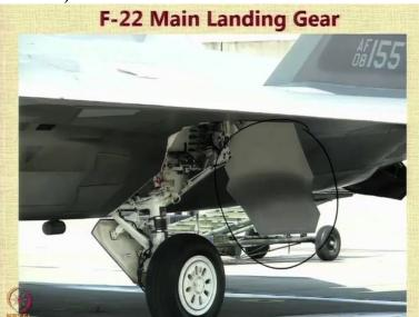
Let us end by looking at some landing gear of famous aircraft and try to familiar ourselves with their functioning. This is the landing gear of the F-22 aircraft. You can notice here that the landing gear is short and compact and as it retracts inside, you have this conformal cover that will fit into the geometry and make the whole aircraft fuselage very much smooth to avoid darg.
