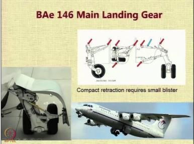
On a BAe 146 aircraft, you have to provide landing gear on the landing gear on the fuselage because it is again a hiding aircraft and when you have turbo fan engines mounted on the wing, then mounting the landing gear on the wing becomes a serious problem what we saw in is an exception, so in this case, you have the landing gear mounted on the side of the fuselage, but you need to have minimum some minimum wheel tracks so that you can get the when you can avoid the tip off.
