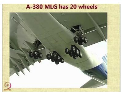
This is the landing gear of Airbus 380. You can see that there are 4 main legs there are 2 on the fuselage on the sides and there are 2 on the wings. So there are 20 wheels in total. There are 6 wheels on each of the main legs on the fuselage, so 12 wheels here and then there are 4 wheels on the main landing gear leg which is in the wing. So, on each side you have 6 + 4. That means you have total of 20 main landing gear legs, and then you have the nose landing gear also which has 4 wheels.
