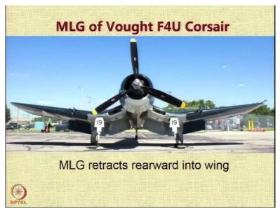
Let us look at the landing gear of an aircraft called as a Vought F4U Corsair this particular aircraft had engines embedded in the root of the you can see there is some intake here and in this case the main landing gear retracts rearward into the wing so it goes back.
