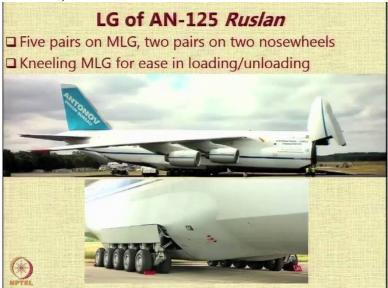
If you look at the landing gear of AN-125 Ruslan aircraft, this is a very interesting aircraft. It is a cargo aircraft for transporting cargo over long distances. So the nose of the aircraft completely bends up. And you have as you can see 5 pairs of landing gear legs on the main landing gear and on the nose wheel; you have 2 pairs on 2 nose wheels. Now, this particular landing gear, we can adjust the length of the struts so that the aircraft can be made to kneel
