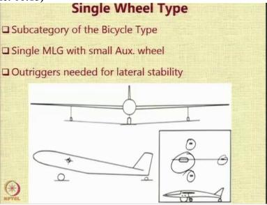
We also have a single wheel type which is basically a subcategory of the bicycle type in which you have just a single auxiliary single main landing gear wheel and a small auxiliary wheel on the back. Again you need outriggers for stability as shown in this particular figure. So, 1 main wheel, 2 outrigger wheels and a small auxiliary wheel for longitudinal stability of the aircraft during operation. Such consideration is very common in gliders.
