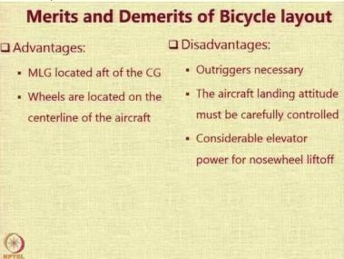
There are many merits and demerits of bicycle type layout. The advantages are that the main landing gear is located after the CG and the wheels are located on the aircraft center line. So
