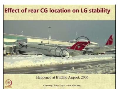
Effect of rear CG location on the landing gear stability is very important as this picture from Buffalo airport shows because of collection of iec on the rear part of the aircraft and loading of the aircraft, you know the tail of the aircraft has hit the ground.
