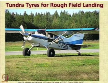
Then when we are want to operate at very unprepared and remote locations, where you have very rough field, you know, we have to provide very special features in the aircraft. This is one example of tundra tyres for rough landing. And these are basically oversized tires with very low pressure and they allow you to operate.
