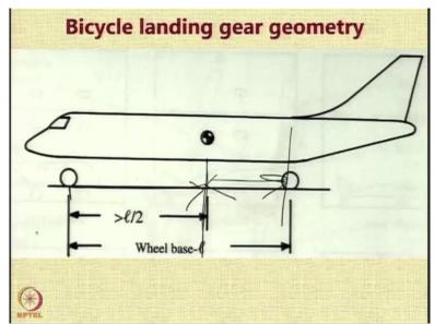
In the bicycle type landing gear, the geometry is such that to allow a little bit easy in the rotation, you keep the centre of gravity more than half the length. So this distance is generally around 35 to 40% compared to these distance. This allows ease in rotation.
