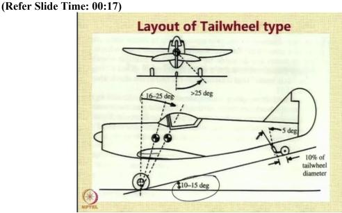
Here is another picture that shows the layout of the tailwheel type which has to be kept in mind while designing a tail dragger or a tail wheel type aircraft. Notice that the 10 to 15 degree angle that might be encountered during take-off has to be considered in locating the landing gear ahead of the centre of gravity with a little bit of margin.
