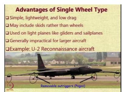
And in many cases, the single wheel type allows the gliders. So these are simple lightweight and low drag aircraft because there is only one main leg, but instead of introducing the wheels you may also have skids and very commonly seen on light planes like gliders and sailplanes. But generally such configurations are impractical for larger aircraft. One example of this particular type on a large aircraft was the U-2 reconnaissance aircraft.
