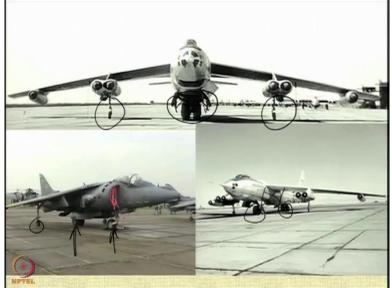
There are some examples of bicycle type. This is one example B 47 aircraft in which the central part of the fuselage where you normally mount the landing gear is occupied in carrying bombs a large amount of bombs and hence the landing gear had to be moved outside. So that is there are 2 main wheels in the front, 2 on the back. And there are outrigger wheels on the sides.
