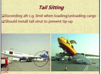
Similarly, there is something called as tail sitting when you exceed aft c.g. limit, while loading or unloading of cargo, you can have this problem in which you know, the rear of the aircraft hits the ground. The one that you saw earlier was because of weather conditions here it is because of improper procedure followed or not following the SOP during the loading and unloading of the cargo. So, as a result, the rear part of the aircraft became heavy and so, the tail has sit on the ground.
