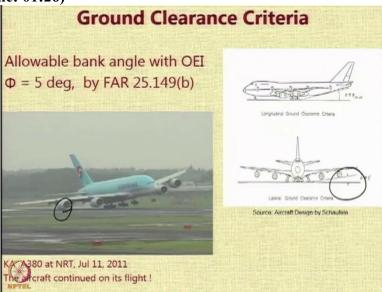
Also it is important to realize that when you design the landing gear, there is a ground clearance criteria. So as per the FAR regulations, if FAR part 25 regulations, when an aircraft comes into land with one engine in operational, we have to allow for a bank angle of 5 degrees. So, the, the landing gear should be located so that even when there is a bank angle of 5 degrees, that wheels do not touch the ground, the engine does not touch the ground.
