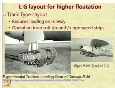
Then taking this particular thing to the extreme, we have track type layout, which reduces loading on the runway and allows the aircraft to operate from soft ground and unprepared strips, just like we have tanks, which have these tracks, you can actually you know load you can actually create a landing gear where you can have track tank like tracks on the ground.
