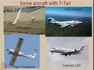
Here are some aircraft, popular aircraft, which have a kind of a T tail configuration. It is a very popular configuration amongst gliders. One of the most efficient riders available today's the ETA glider. You can see how much the wing is flexing in the flight. And that configuration has a T-tail. Piper Tomahawk is another famous aircraft which has a T-tail. And there are other 2 aircraft, the military F-101 voodoo and the Canadair CRJ, they all have a T-tail configuration.
