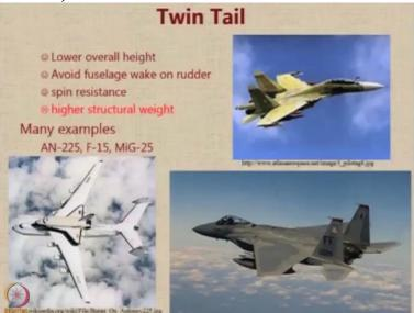
Twin tail is very common in military aircraft. Generally a twin tail is given if you would like to reduce the height of the tail. So instead of one big tail you can put 2 tails and also it helps
