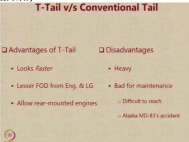
Let is compare a T-tail versus a conventional tail the detail looks faster, because it is far away, it will be less prone to foreign object damage from the engine and the landing gear and
