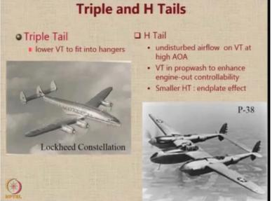
Then we also have triple tail and H tails. Lockheed constellation is an example of a triple tail configuration and this is a need driven by the requirement to fit the aircraft vertically into the hangar which are available. The horizontal the H tail has undisturbed flow on the vertical tail at high angle of attack, this is the H tail configuration in the P-38. So, what you do literally is you move away the vertical tail from the wake of the engine and also you provide double tail configuration.
