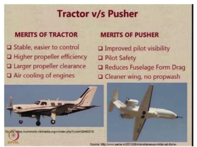
Let us have a look. Let us first look at the merits of the conventional configuration or the tractor configuration. The first and the most important factor is that a tractor configuration of engine gives you a configuration that is stable and relatively easier to control. Because the propeller is in undisturbed flow facing the wind as the aircraft flies forward, you get higher propeller efficiency.
