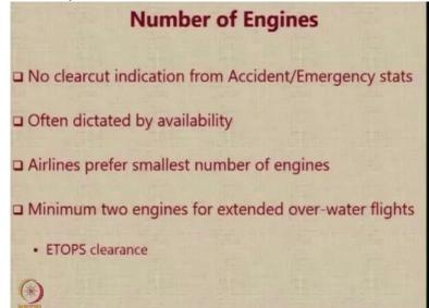
As far as number of engine is concerned, there is no clear cut indication from any accident or emergency statistics that have been equal number of accidents when their craft is with 2 engines or with 3 engines or with 4 engines. So, having more engines more than 1 see more than 1 is essential because you need to have redundancy and therefore, you need to have at least 2 engines especially when you carry a fair amount of passengers.
