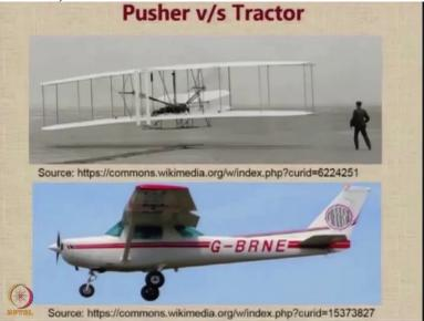
So, when we look at the engine location, the first choice that we are encountered with is whether to use a pusher configuration or a tractor configuration. The pusher configuration is very, is considered today as uncommon and special. But interestingly, the first aircraft to fly successfully, the Wright flyer of 1903 was a pusher configuration and most of the aircraft which are used today that are meant for training of pilots or general aviation.
