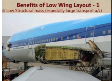
Finally, we come to the low wing configuration such as the one in this spit fire aircraft. The first benefit of a low wing layout is that it leads to lower structural mass and this becomes extremely important and relevant, when we look at large transport aircraft such as the airbus A 380 or the Boeing 787. In these aircraft, it has been shown that lowing configuration leads to the least possible structural weight.
