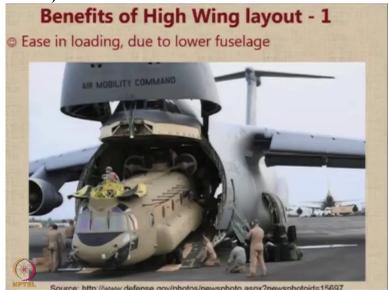
The first and foremost benefit of a high wing layout is to permit ease in loading and unloading of cargo because the wing is mounted above the fuselage; hence the fuselage height tends to be low. This is a very good example of a military cargo aircraft.
