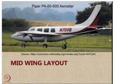
Let us move on to the mid wing layout. The mid wing layout is a layout in which as we can see in this Piper PA-60-600 aerostar the wing is mounted in the center of the fuselage.
