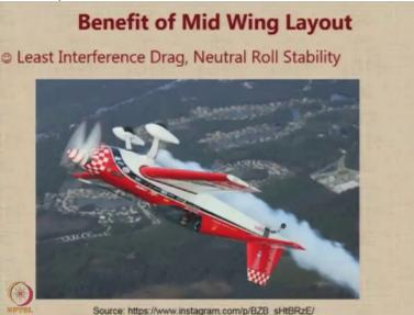
Now, the most important advantage of a mid wing layout is the aerodynamic advantage. A mid wing aircraft has the least interference drag and also it has neutral stability. These parameters make it the configuration of choice for all aerobatic aircraft in most fighters and aerobatic aircraft, we observed that we go for a mid wing layout.
