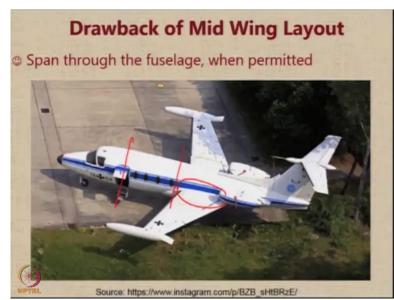
However, a mid wing layout leads to a restriction on the design of the carry through structure and the spar because in normal circumstances in a mid wing aircraft, the spar carried through structure will go through the fuselage and that will create a lot of trouble or the disturbance in the passenger cabin. One solution for such a problem is to have a configuration in which the entire passenger cabin is ahead of the wing such as the one in this Hansa jet aircraft.
