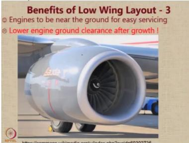
But then, when you go for changes in the fuselage length, when you go for upgrades of the aircraft, the same low wing location which gave an advantage of engines nearby become a problem because as in this case, this is an example of the same Boeing 737 aircraft, but now this is dash 600 version the 600 version had more the CFM 36 engines, which were more efficient than the GTA DS which are used earlier in dash 100 and dash 200 engines, but these engines were larger in size.
