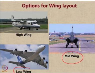
So, these are the images of some famous aircraft which have these configurations. The high wing configuration shown here is the Dornier 228 dash 212 aircraft which was produced under license by HAL Kanpur.
