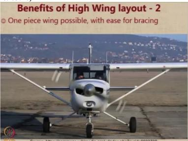
One more advantage of a high wing layout is that you can build the whole wing in one piece and then put it literally over the fuselage, attach it with some bolts and you can externally support it by using braces such as the one seen in this aircraft. So, this gives a huge structural advantage and results in a light weight structure.
