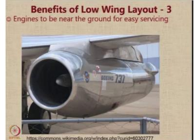
A low wing configuration also allows mounting of engines in the proximity of the ground, and hence for the maintenance crew. It is very easy for them to look after the engines or to do the inspection and the maintenance activities such as the case in this photograph of a Boeing 737 dash 100 aircraft.
