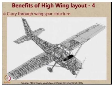
This is an example of the mounting of the high wing, you can see that you can have a through and through spar. As you can see here, the spar can be through the rear spar and this is the front spar. Both can be through and through. And that leads to tremendous structural advantages.
