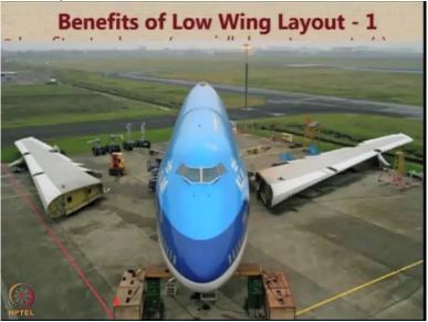
This is another photograph of the same aircraft which shows the 2 wings being brought in for assembly at the location.
