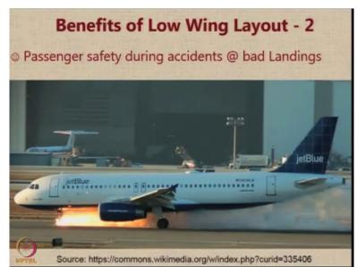
One more benefit of the low wing layout is it gives you additional safety during accidents. In case there is a bad landing, in which let us say the landing gear is crumpled or there is a tyre burst. Or as in this case, when you see for a JetBlue aircraft there was in a locked nosewheel and it was actually turned sideways. And when the aircraft came in to land, the nosewheel tyre actually was so hot that the nosewheel caught fire.
