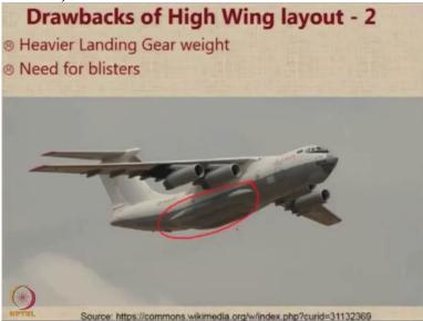
And when the aircraft takes off and the landing gear is retracted, there is a requirement for these large blisters on the fuselage and these blisters create additional drag and also additional weight.
