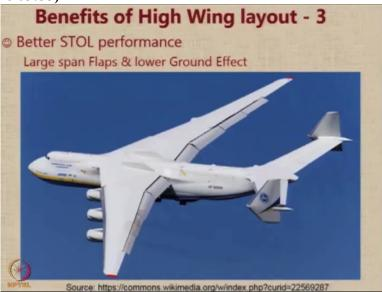
The third benefit of a high wing layout is to allow better short take-off and landing performance, because we have a huge uninterrupted wing mounted over the fuselage, you can have flaps over a much larger span and since you are away from the ground, you will also be
