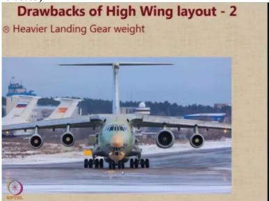
Another drawback of the high wing layout, which I discussed a few minutes ago is also due to the landing gear being heavy, the landing gear is heavy because the landing gear cannot be mounted always on the wing, you can see the landing gear is mounted here along the side of the fuselage, you need to have a sufficient amount of wheel track for stability in the ground motion.
