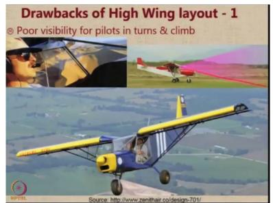
One serious issue of concern for a high wing is poor visibility of the pilots especially when they go into turning and climbing flight. As you can see here, the port side view of this pilot is obstructed to a large extent by the presence of this particular wing structure. Now, special features have to be provided in the aircraft. For example, you can see in this aircraft, they have actually created a cut in the wing at the root and on the top of the fuselage canopy.
