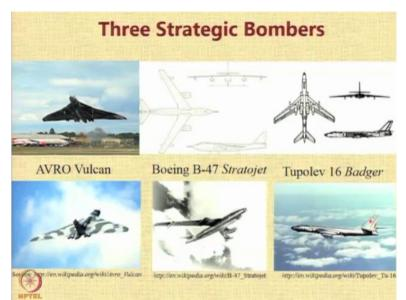
On the extreme left is the flying wing configuration of AVRO Vulcan bomber. In the middle, is the Boeing B-47 stratojet, which is a conventional configuration with a highly swept wing. This is from the American designs table. On the right, is the Tupolev 16 Badger, which is a solution to the same problem by the Russians. So we noticed that to meet the same requirement or almost similar requirements of a strategic bomber.
