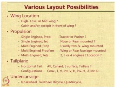
So when you look at the layout of the aircraft, you have various possibilities. First, let us look at the possibilities for the layout of the wings should we go for a high wing that means the wing mounted over the fuselage, should we go for a low wing, the wing mounted below the fuselage or should we go for a mid wing should the passenger cabin and or the cockpit be located ahead of the wing in the middle of the wing or behind the wing.
