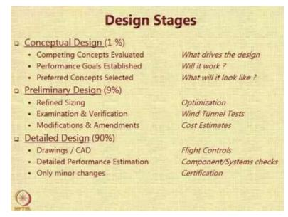
These particular stages are actually the same as what we saw in the previous clip regarding the phases in aircraft design it is just a different way of looking at the same thing. So the first stage of aircraft design is the conceptual design stage which involves only 1% of the total effort involved in aircraft design. In this there are few activities we do, we look at competing concept and we evaluate them.
