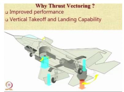
So, this is how it works, there is a dedicated lift fan in the front portion of the aircraft which is normally covered in the normal flight or in the forward flight it is covered by these cowlings and these bottom cowlings and there is also a duct which is going to create 2 jets of air coming out from the main engine and the nozzle of the engine the rear of the engine is also swivel down.
