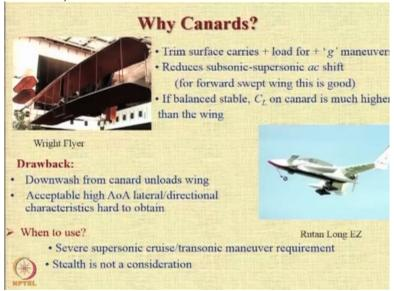
Another feature that we would like to understand is a canard, a canard is basically a tail mounted ahead of the aircraft rather than a conventional tail mounted behind. One of the advantages of providing a canard is that the trim surface or the canard carries a positive load for positive g maneuvers and that helps in reducing the load that the wing has to carry. Secondly a canard reduces the subsonic supersonic aerodynamic centre shift.
