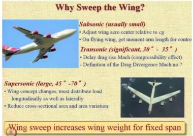
One question that many people ask is why sweep the wings, what is the benefit of providing sweep back on the wing? When it is a subsonic aircraft usually we provide a very small amount of sweep 1 reason for this could be to adjust the wing aerodynamic centre relative to the centre of gravity, because, you would like to have the distance between them the minimum.
