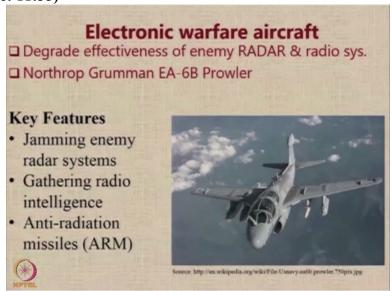
We also have some aircraft which are meant for electronic warfare so their aim is to degrade the effectiveness of enemy's radar and the radio systems. One example is the Northrop Grumman EA 6B Prowler aircraft. So you can see the key features of this aircraft are to jam the enemy radar systems, they gather radio intelligence and they also have anti-radiation missiles.
