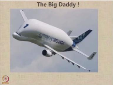
Here is the big daddy the Airbus Beluga, which was designed essentially to carry large sub-assemblies fuselage of the Airbus aircraft for final assembly at Toulouse.
