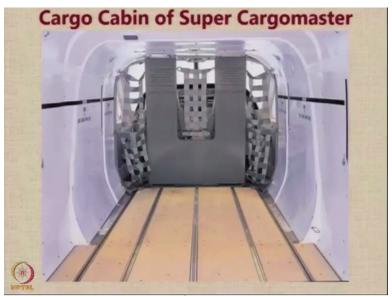
Just to give you an idea here is the cargo cabin of a super cargomaster, there is a partition which protects the crew from the movement of the cargo and you will notice that the fuselage has got this very high strength floorboards and the seat rails and these seat rails are having notches at every approximately 1 inch location. So, you can actually adjust the equipment at any particular point along the length of the fuselage.
