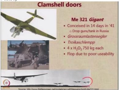
Going back to history, we look at one aircraft called as the Messerschmitt Me 321 gigant which basically means giant. This aircraft was conceived in a period of only 14 days over 2 weeks in 1941 during the Second World War, and the aim was to design an aircraft which can quickly be used to drop guns and tanks in Russia when the German forces were fighting the Russians. So, this is basically a grossraumlastensegler which in German means a large sized long range glider.
