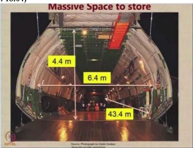
And the wingspan of the aircraft is 88.4 meters. And if you look at the cargo cabin, you have a height of 4.4 meters or width of 6.4 meters and a gross length of around 43.4 meters available for you to carry the cargo. So, this is a real heavy lift aircraft.
