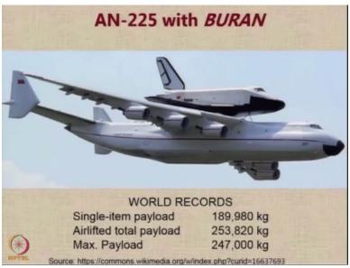
And the main design requirement for this aircraft was to carry the Russian Space Shuttle called Buran. So you can see in this picture, the space shuttle from Russia mounted on top of the aircraft being transported. As I mentioned, there are many world records in the name of AN225 Mriya as far as payload is concerned. So you can see some numbers around 190 tons of payload. Single item 250 odd tons total airlifted payload 247 tons is the max payload that can actually be mounted.
