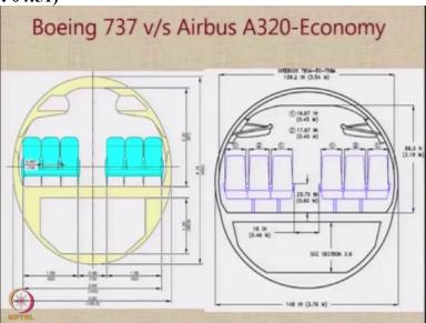
Here is a comparison of the cross section of Boeing 737 versus Airbus A320 we noticed that the both the aircraft have a 6 abreast seat layout and a clearly compartmentalized fuselage and the dimensions are also quite similar.
