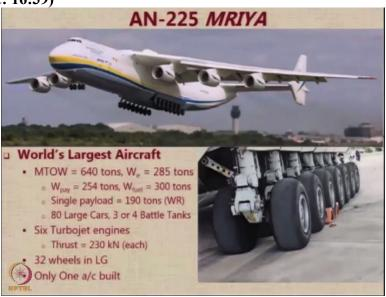
Here is the world's largest aircraft, is AN225 MRIYA which is a dedicated heavy lifter. This is the world's largest aircraft, it weighs 640 tons the max takeoff weight and it can carry a payload of 254 tons on an empty weight of 285 tons and it carries 300 tons of fuel because there are 6 engines. So there has been a world record of a single payload of around 189 190 tons. It can carry 80 large cars, 3 or 4 battle tanks. Each of the engines produces a thrust of 230 kilo Newtons.
