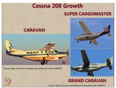
So this is the Cessna caravan the basic aircraft caravan 1. You can see that it has these passenger windows and high wing layout with the based wing. On the bottom we have a fuselage shape to carry certain items in the belly, the super cargo master is the one in which the windows are completely removed everything else remains and you actually fill up the whole aircraft with cargo and from super cargomaster, again a reverse version of a passenger aircraft was created called as the Grand Caravan.
