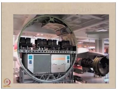
Here is a cross section of a larger Airbus aircraft, where you can see the top cabin has a seating of 8 abreast and on the bottom we have these containers they are called as the LD3 containers, containers to be carried on the aircraft come in various sizes and there are there is a dedicated series LD3 LD4 etc. So, there are these dedicated containers which are designed keeping in mind their transportability below the belly or in the belly of transport aircraft.
