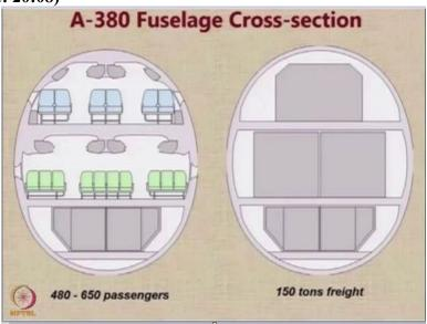
Here is a cross section of Airbus A 380 when it carries passengers, as we know the Airbus A 380 is an aircraft that has twin passenger cabin along its entire length. It is a double decker aircraft
