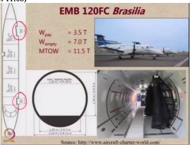
Another example of a popular aircraft which is a passenger variant into a cargo is the EMB 120 FC Brasilia, this aircraft has a payload of 3.5 tons on an empty weight of 7 tons and the max takeoff weight is 11.5 tons. So, you can see in this aircraft, the whole of the fuselage is meant for only carrying the cargo and in the center of the fuselage there is a floor with mounted with these
