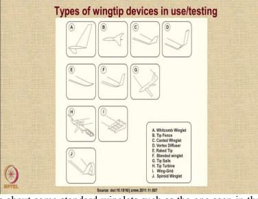
All of us are aware about some standard winglets such as the one seen in the top 4 of this slide, the Whitcomb winglet, the tip fence, the canted winglet and the vortex diffuser, but there are some interesting wingtip devices which are under investigation. And we are going to look today at the last one which is marked as J the Spiroid winglet.
