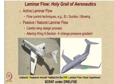
Laminar flow or maintaining laminar flow on an aircraft for a large part of the large fraction of the aircraft surface has been the holy grail of Aeronautics, right from the beginning people have attempted to achieve laminar flow. One way of achieving laminar flow is called as active laminar flow control where we use techniques like boundary layer suction or boundary layer blowing to proactively create laminar flow, but this requires a lot of energy and power.
