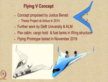
Which is a concept that has been proposed by Justus Benad as a thesis when he carried out his internship at Airbus in 2014. So, once this study was carried out, this concept was taken up by Delft University in Holland and KLM. Now, in the case of a Flying V concept, the passenger
