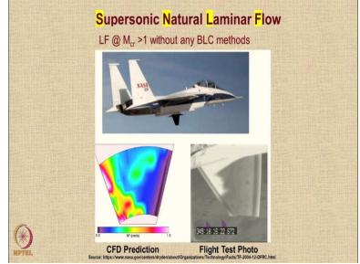
So, that is a huge achievement. So, if you look at how supersonic natural laminar flow is created, basically the aim is to create laminar flow at Mach numbers more than 1 without any active boundary layer suction methods. So, NASA has done a season experiments on a small stub mounted below the fuselage and it was this is a CFD prediction and this is the actual flight test information.
