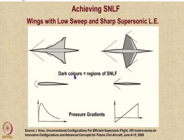
So, how do you achieve supersonic natural laminar flow one mechanism is you use wings with low sweep and sharp subsonic leading edge. So, you can see that this is one possibility, you have low sweep but very sharp leading edge. So, with that sharp leading edge, you get a particular end like this or you could use the conventional approach where it is slowly increased to high value and then comes down slowly.
