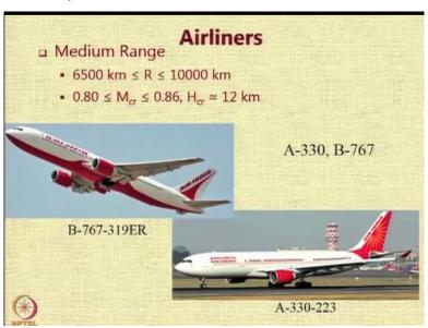
The next category is the medium range airliners which start at 6500 kilometers and goes up to 10000 kilometers. The cruise Mach number does not increase too much. It goes from approximately 0.80 to 0.86 and they may fly at a slightly higher altitude of around 12 kilometers. Obviously, the altitude that you fly is limited by the instruction from the air traffic controller okay.
