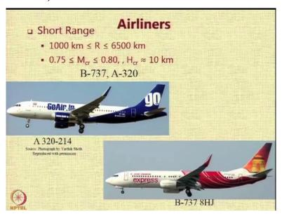
So, in the short range airliners, we normally start from about 1000 kilometers where the long range regions are ending and we go up to 6500 kilometers. Most of these aircraft operate with a cruise Mach number between 0.75 to 0.8 they fly at height of approximately 10 kilometers or 35000 feet above the Earth. Now in this particular category the popular aircraft that we see in India are the Airbus A 320 and the Boeing 737 as you can see in this particular picture.
