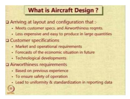
That aircraft design essentially consists of arriving at layout and configuration which can address two things. One, It should meet the customer specifications and the airworthiness requirements and second, it should be less expensive and easy to produce in large quantities. The second point is the one that actually decides to a large extent the choice of materials, the choice of manufacturing processes.
