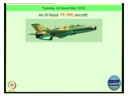
That this is a FT-7PG is a Chinese Aircraft. You can see there are two, what do you see? Two ventral fins are mounted and what about the intake? It is a nose mounted intake. So this is an authorized, licensed version of a Chinese aircraft which was a copy of a Russian aircraft.
