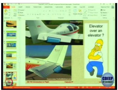
Alright so now the interesting thing is that here you have a Elevator and you have a small deflecting surface over the Elevator. So what is this? A small Elevator on the Elevator. This is a trim tab this
