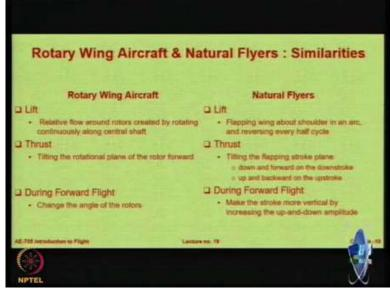
Similarly when you want to tilt, when you want to go forward, you tilt the thrust rotational plane. Same thing is done by the birds and by the insects also, they tilt the flapping stroke plane and that is how they get the forward motion and during forward flight, you change the angle of the rotors. Similarly, you change the angle of flapping. So I would say that the helicopters are actually doing many things just like what the birds are doing.
