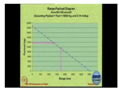
So the blue line that you see is the tradeoff between range and payload and these two purple lines or cyan lines the horizontal one is the cut because of the limitation on the maximum structural weight and the vertical one is the cut because of the maximum fuel capacity of the aircraft and the inclined line in between is the permitted operational tradeoff between range and fuel.
