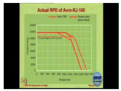
So this is the actual range payload diagram of this air craft from the operating manual from the aircraft manual and these pannier tanks basically are those additional fuel tanks that you can fit inside the aircraft for delivery purposes. So you can see that with 112 passengers at 95 kg each this is your range payload diagram, there is no line it is just increasing.
