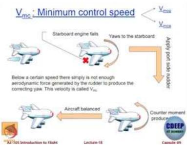
So moving back let us look at V mc. V mc stands for V minimum control or minimum control speed, so to understand this let us watch a short video:
