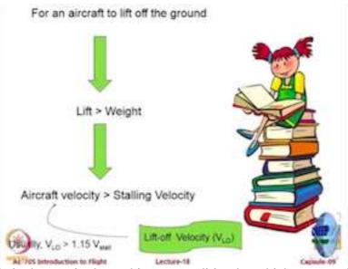
So essentially this is the required to achieve a condition by which you can leave the ground. So what is required for the aircraft to lift off the ground? You require that the lift has to be more than weight, ok. And to get that the velocity of the aircraft should be more than the stalling velocity, ok. But do you think an aircraft can be operated or should lift off just at V stall? Or do you think some margin should be given? It will be unsafe to lift off at V stall.
