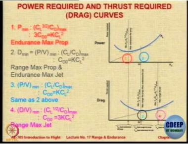
And finally, if you look at the comparison, there are these four speeds. That is one speed, number one at which power is minimum. Therefore endurance is maximum for a prop, there is another speed at which drag is minimum. That will give you the maximum range for props and maximum endurance for jets. Point number three is the same. Point number four will be the range for jets to be maximized.
