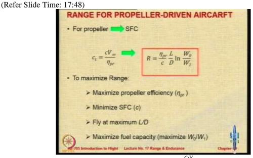
So, for a propeller aircraft we use that relationship  $C_t = \frac{C \cdot V_{\infty}}{\eta_P}$ . So,
