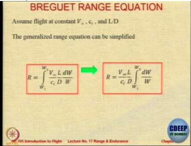
For example, there is one condition of flight in which velocity may remain constant but altitude may not remain constant. Do you remember I talked about cruise climb condition in which as the aircraft is losing the weight, you slowly increase the altitude. So, during that time this cannot be acceptable because Ct will not remain same, as density changes Ct will change.
