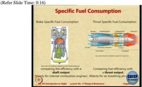
So, let us look at what exactly determines how much you can travel on a given amount of fuel and that one of the important parameter is the SFC. So, for an IC engine it is the brake specific fuel consumption and for a jet engine is TSFC, so in the brake in the BSFC or in the IC engines we are concerned about the break or the shaft horsepower. Here we are concerned about the thrust produced directly.
