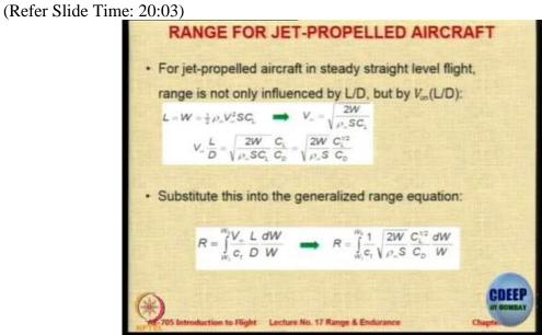
For a jet propelled aircraft the only influence is L/D. So, one can easily derive the expression. So, it is very messy it is not a very simple expression. So L/D alone is not important because V also is there, so you have to optimize V, L/D.
