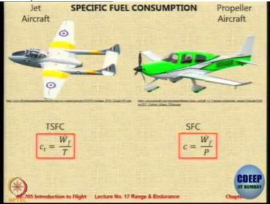
So, for jet engine aircraft we talk about TSFC or the thrust specific fuel consumption called as  $C_t = \frac{\dot{W_f}}{T}$ . For propeller aircraft we are concerned about power so we define SFC as the fuel flow per unit power produced.
