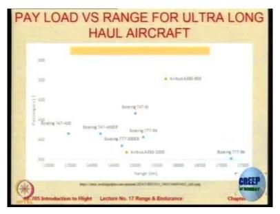
So you can see now there are some ultra long aircraft. So there is this Boeing 777-8X which is made into Boeing 777-9 you can see the range is 17,250. So many aircrafts are available who can fly but the payload is the lowest, it is just 350 passengers and Airbus 380 is here it can travel around 15,500 and more but it can carry 555 passengers.
