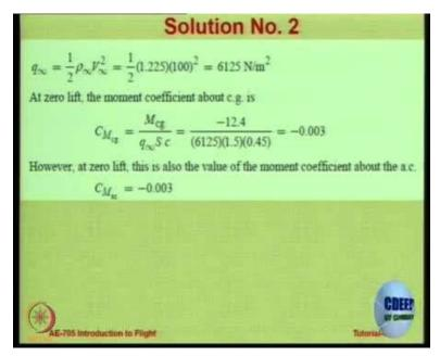
Okay. So, the first thing you can do is to calculate dynamic pressure which is half into rho infinity into v infinity square. Since, the conditions are sea level density is 1.2256 or 1.225 kg per metre cube and the velocity given is 100. So, this is the dynamic pressure.
