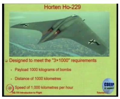
This is the most famous of their flying wings Horten-229 and this aircraft was designed to meet the requirements of 1000 by 1000 by 1000 which was proposed by the German Luftwaffe in almost at the end of Second World War. So, the requirement was to carry 1000 kilograms over 1000 kilometres on 1000 kilometres per hour.
