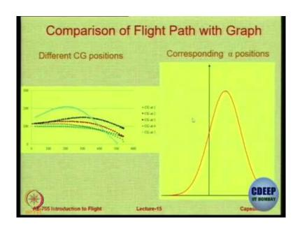
So this is a graph of the L by D verses alpha. So, at alpha one we had some angle of some L by D. At alpha two we had some L by D. at alpha three we had the best L by D at Alpha Four we had less, Alpha five was the worst. So that is why at three I get the maximum range. So, on the left hand side we have the flight flight profiles on the right side we have the corresponding Alpha positions, Yes.
