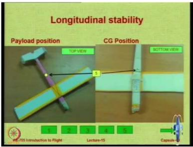
So, let us see. So, this is the glider that was made. You have a top view and a bottom view. In the bottom view we have drawn some lines. These lines are the location of some payload that we have put to adjust the center of gravity. So, this aircraft will have some center of gravity location on it is own because of its geometry. But if you want to play with the CG you have to add weight.
