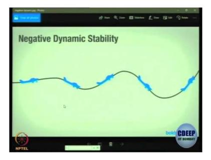
In neutral once again, the oscillations are same in the magnitude in the in the amplitude when you disturb the aircrafts it oscillates, but it does not either come down or go up it remains. This is neutrally stable. It is stable because it is not unstable. That's why we says stable and obviously unstable or negative stability is when, the oscillations are going to worsen increase further with time.
