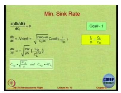
But suppose for example, a situation where theta is very small, which is normally the case in the case of gliding okay, so now we want to find the condition at which what should be the  $C_L$  and hence what should be the V? Because the V and  $C_L$  are connected to each other, what should be the  $C_L$  at which I get the maximum sink rate? And I am assuming that  $cos\theta$  is almost equal to 1.
