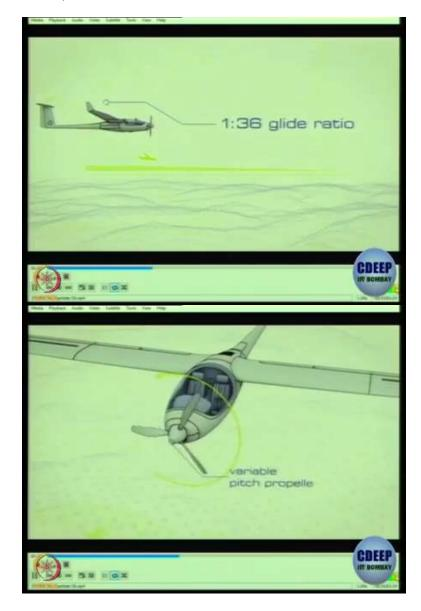
So here is again one of the best motor gliders available today is this one. This is with the engine 1593 kilometers with the engine so glide ratio means L by D, L by D is 36 in glide, this is a sales video which says that you can do so many things, you have so many choices.
